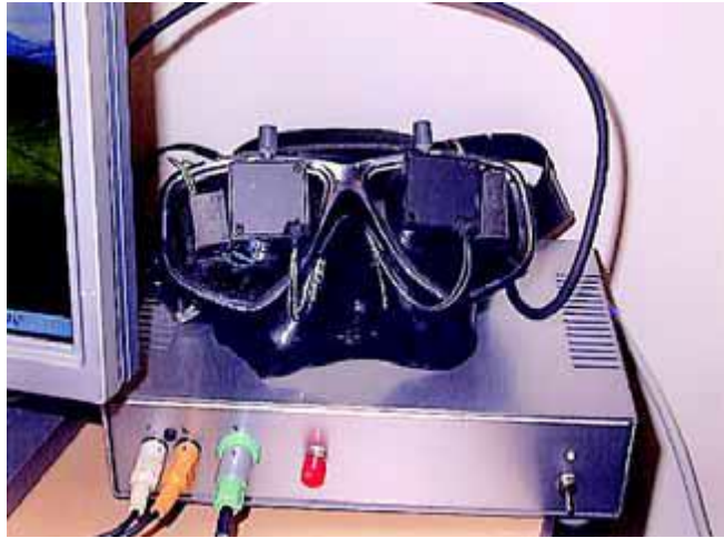
Figure 2. 3: Eye tracking system composed of a head-mounted goggle and control box
