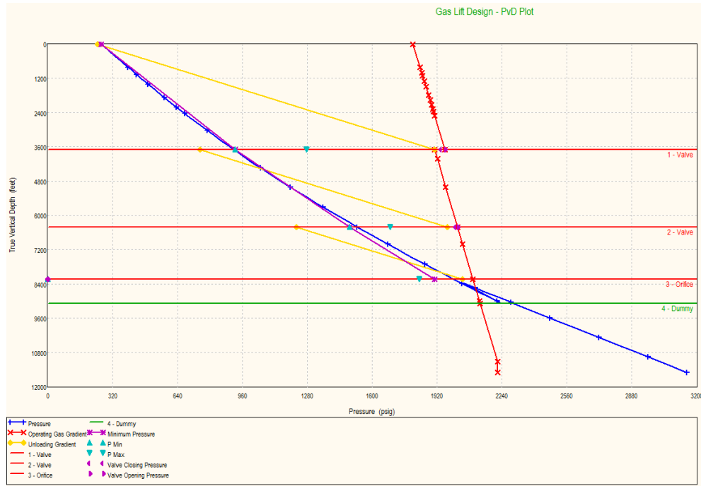
Figure 5.29: Gas lift design: PvD plot (Case 4)
