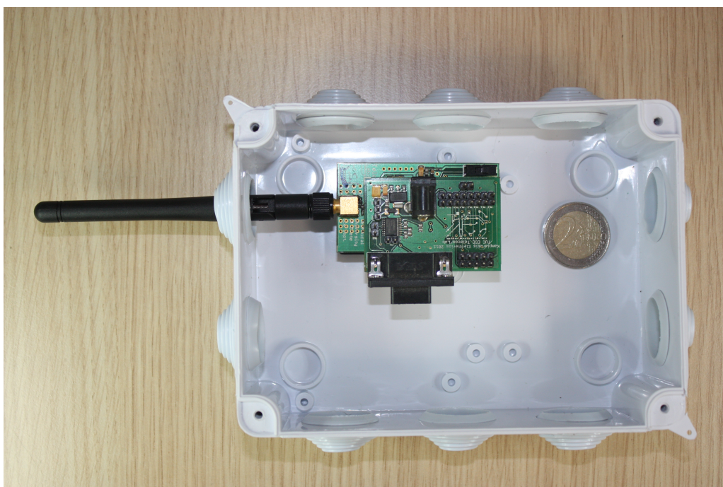
Figure 4.1: An icube, the node used in the implementation, shown in ip64 casing.
