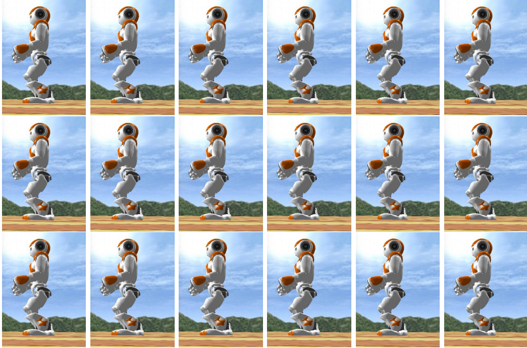
FIGURE 5.2.5: Two steps of the walking behavior with known parameters from the first optimization experiment \epsilon = 0.76319 , \eta = 0.8458 , \gamma = 8.0 , \mu = 1.0 and fitnessfunction = 1.3919 .
