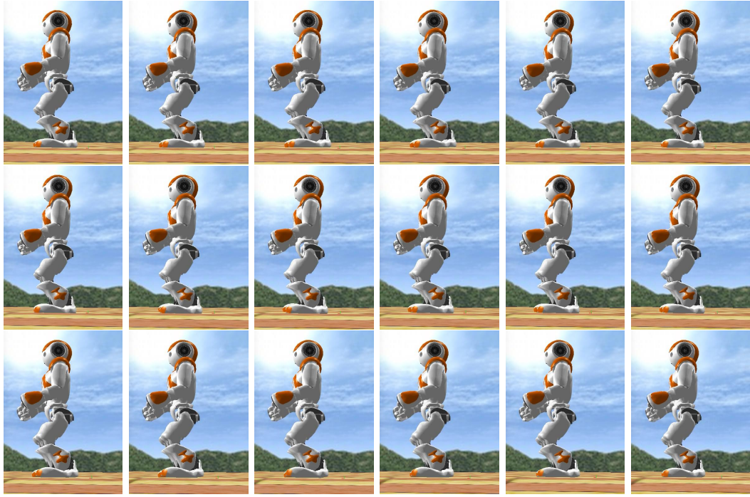
FIGURE 5.2.6: Two steps of the walking behavior with the best fitness function's Ga result with parameters \epsilon = 2 , \eta = 0.96229 , \gamma = 0.43712 , \mu = 0.31136 and fitnessfunction = 2.8318 .
