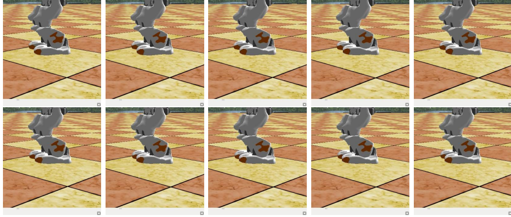
FIGURE 5.2.4: One step of the walking behavior with random parameters \epsilon = 0.55465 , \eta = 0.65465 , \gamma = 0.65749 , \mu = 0.24194 and fitnessfunction = 69.4963 at the begin of the second optimization experiment.
