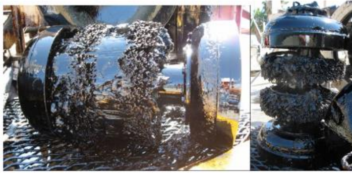
Figure 46: Pig after remedial work on a pipeline
