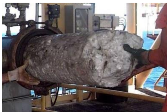
Figure 10: Hydrate plug inside a pipeline
