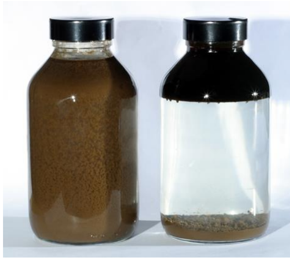
Figure 7: Water/oil emulsion and separated phases after enough retention time
