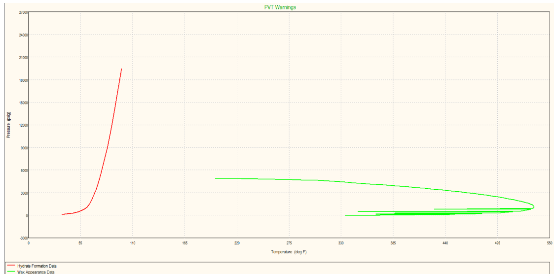
Figure 75: Hydrate dissociation curve and gas condensate phase envelope
