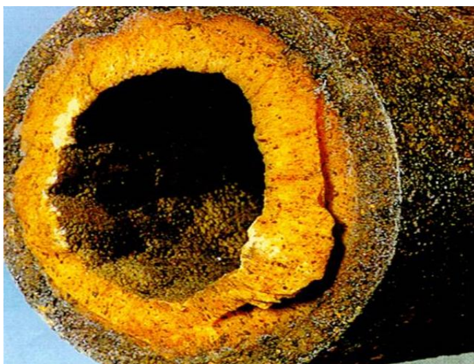
Figure 4: Paraffinic wax precipitation on the pipeline wall
