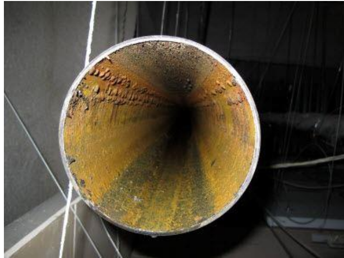
Figure 6: Internal view of a corroded oil pipe
