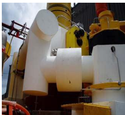
Figure 39: Silicone-based Syntactic Insulation
