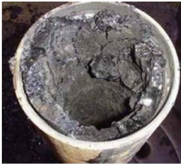
Figure 5: Asphaltene deposition on the pipeline wall
