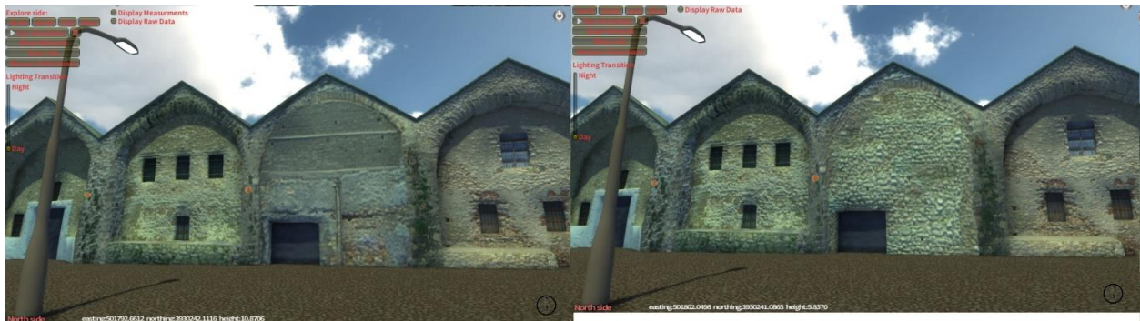
Figure 6.12 On the left added cement can be seen on the monument's facade. The user can toggle between materials in order to visualize the original surface.
