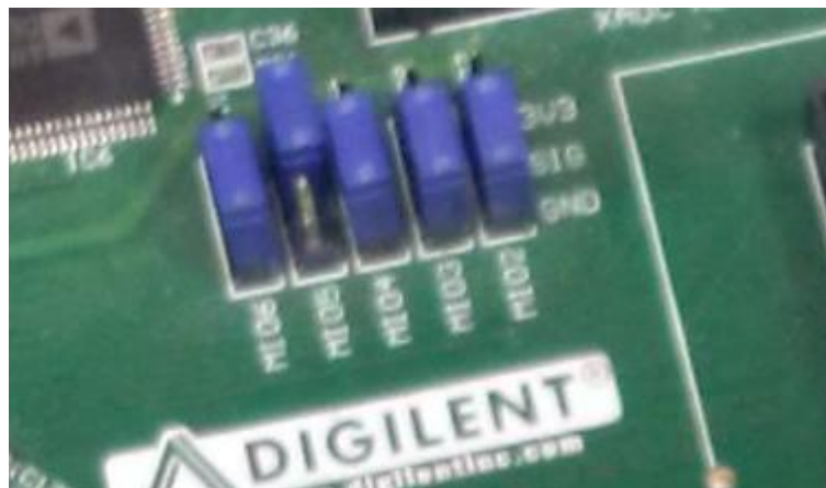
Figure 26 - Jumper position for SD card booting
