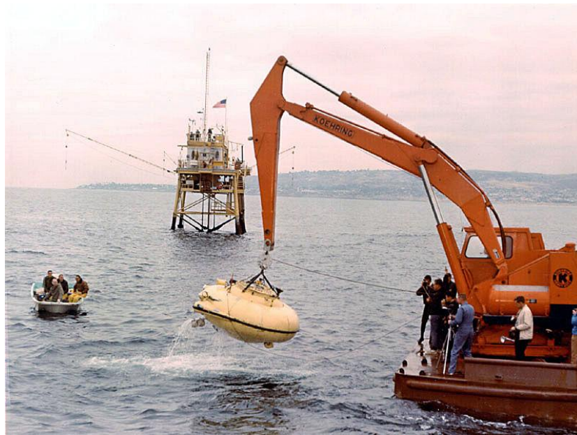
Figure 5 - "Diving saucer," an experimental underwater vehicle that could reach a depth of 350 meters
