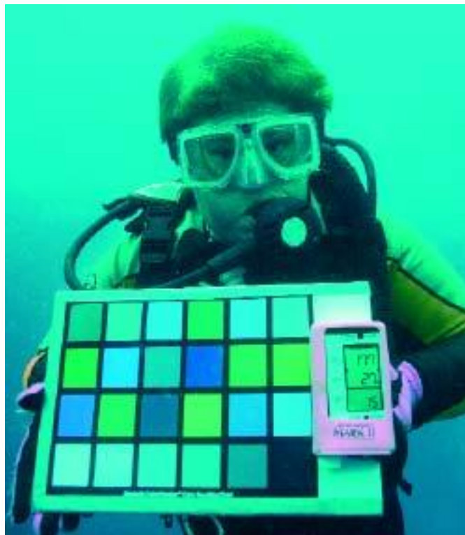
Figure 26 - Digital image with a test chart designed to measure the different levels of colour falloff at various depths
