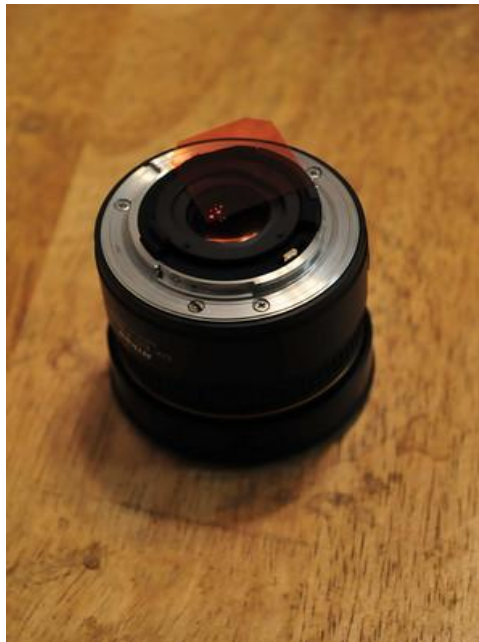
Figure 55 - An example of a red (650nm) colour filter
