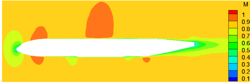
Figure 7.68: Predicted Mach number contours on the symmetry surface of the aircraft (turbulent flow over the CRM WB aircraft).
