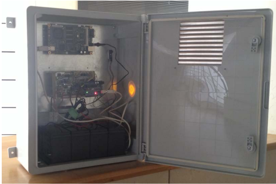
Fig. 21. The interior of the IP65 box with all electronic systems installed and in operation.
