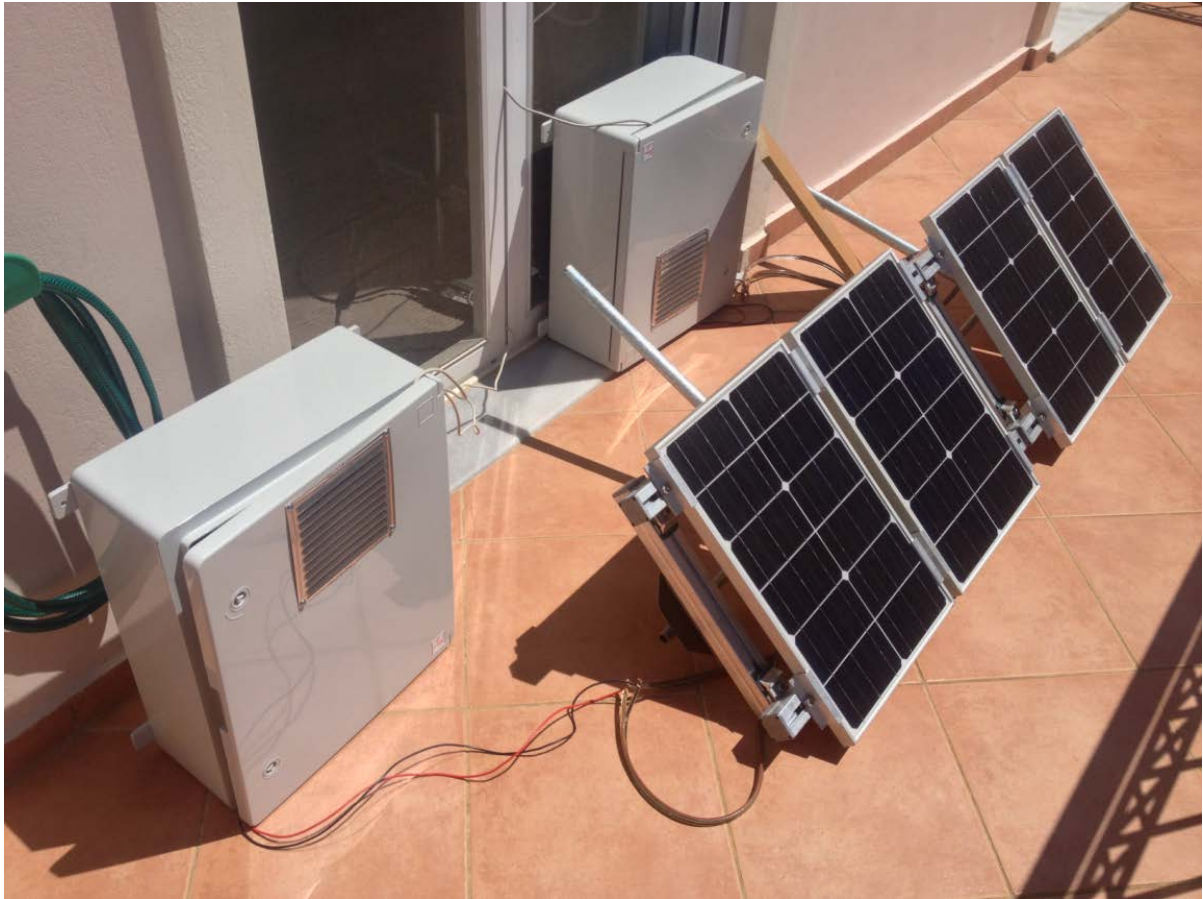
Fig. 22. Two of the prepared stand-alone systems as they were placed during the preliminary operation tests.
