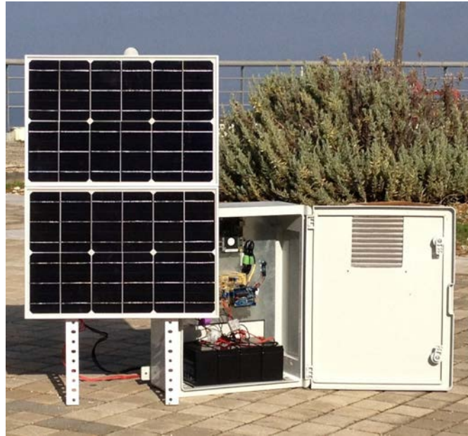
Fig. 24. The experimental prototype of the WSN node power-supply system, which has been designed according to the proposed optimization technique.
