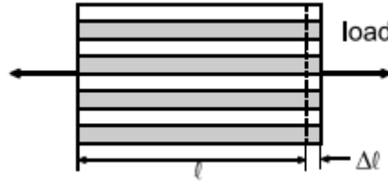
Figure 5-11 A simple unidirectional composite lamina under tensile load [23]
