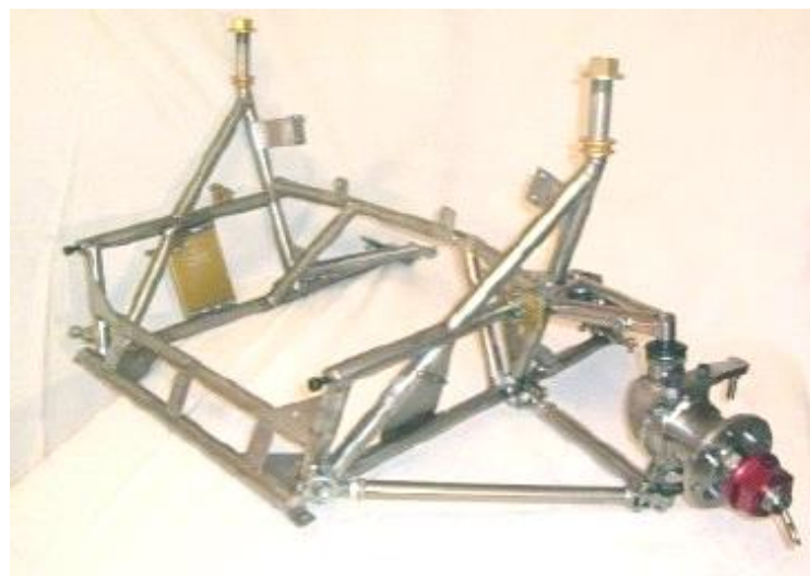
Figure 2-38 Front subframe
