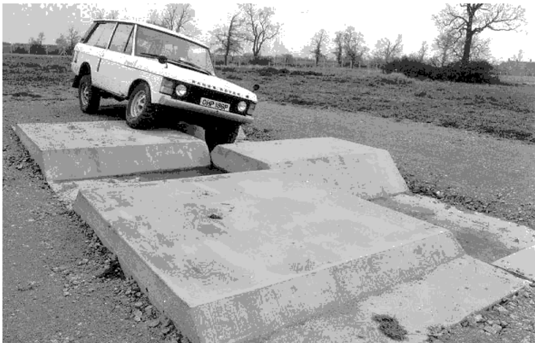
Figure 8-29 Vertical asymmetric (“pure torsion”) load case (courtesy of National Motor Museum, Beaulieu) [2].
