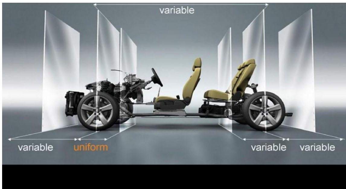
Figure 2-37 The MQB Platform [6]
