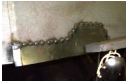
Figure 2-58 Stitch welding
