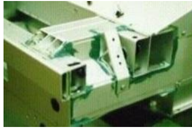
Figure 2-24 Lotus Elise tub chassis design made from glued-together aluminium sheet [5]
