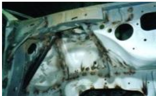
Figure 2-69 Welding Improvements
