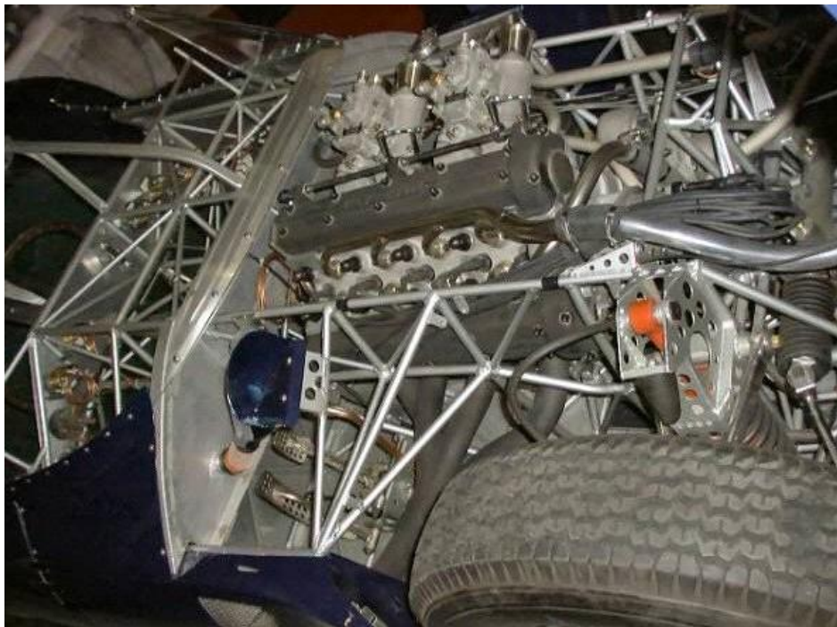
Figure 2-16 Maserati "Birdcage" chassis [2]
