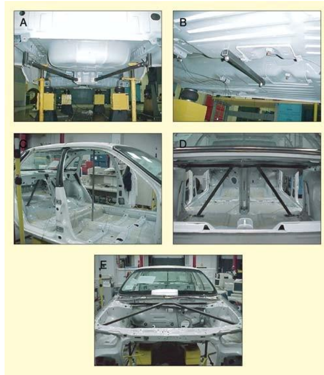
Figure 2-70 A – quad box to rail support, B – tunnel strap, C – floor to roof pole, D – rear shocks to rear floor support, E – front shock to radiator support [8]
