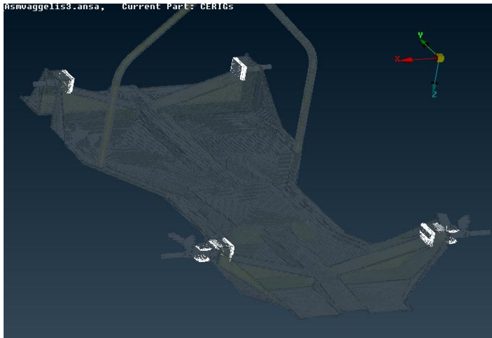
Figure 11-48 Contact Flanges on the Monocoque Chassis (View 1)
