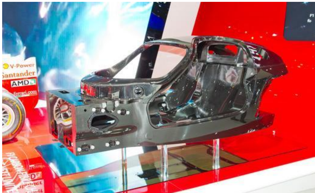
Figure 2-30 Enzo Ferrari Chassis
