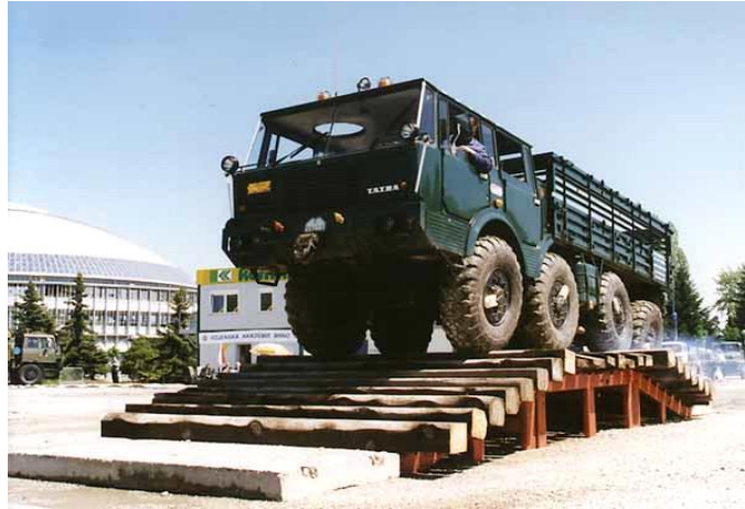
Figure 2-21 Tatra used a backbone chassis on large military trucks
