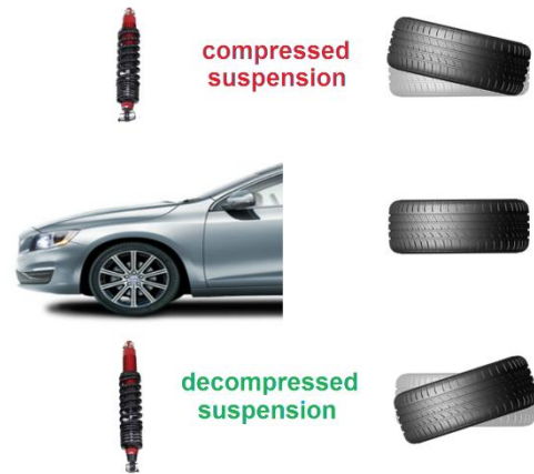
Figure 13 – Illustration of Roll steer. Usually on modern vehicles, when the suspension is compressed the tire tends to steer towards the centreline of the vehicle.
