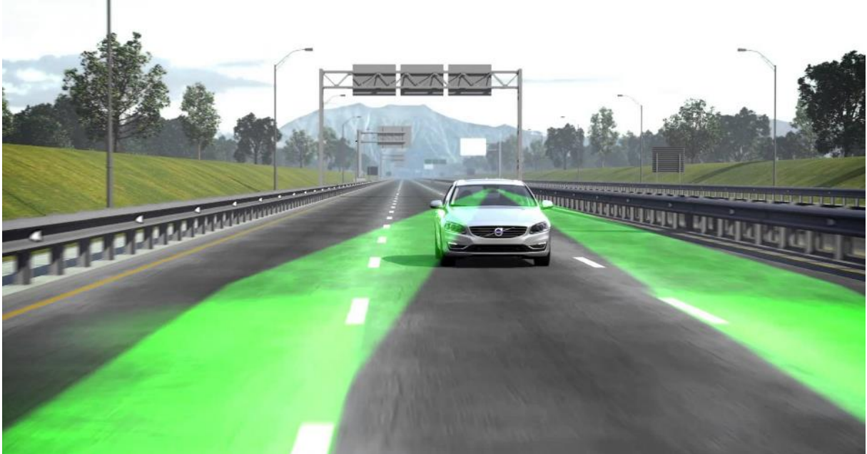
Figure 39 - Illustration of a LKA system. The vehicle identifies the road lane markers using optical sensors (camera) and acts on the steering to correct the path if the vehicle is about to move out of its lane.
