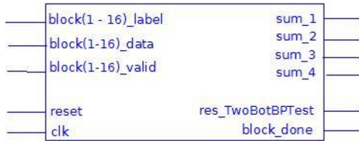
Figure 2.2 Computation Core Block Diagram
