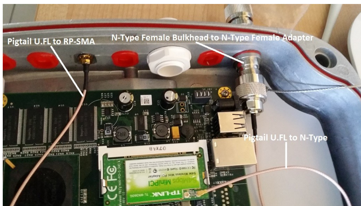
Figure 36: Connectors used in box (inside view)
