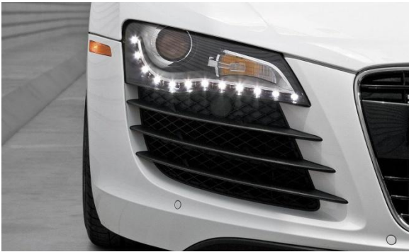
Figure 34 – Mid-range LEDs used in automotive light.
