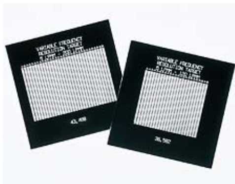
Figure 7.14: The Target we use to evaluate resolution of the Spectral Imager: Edmund Variable Frequency Target #43 – 488
