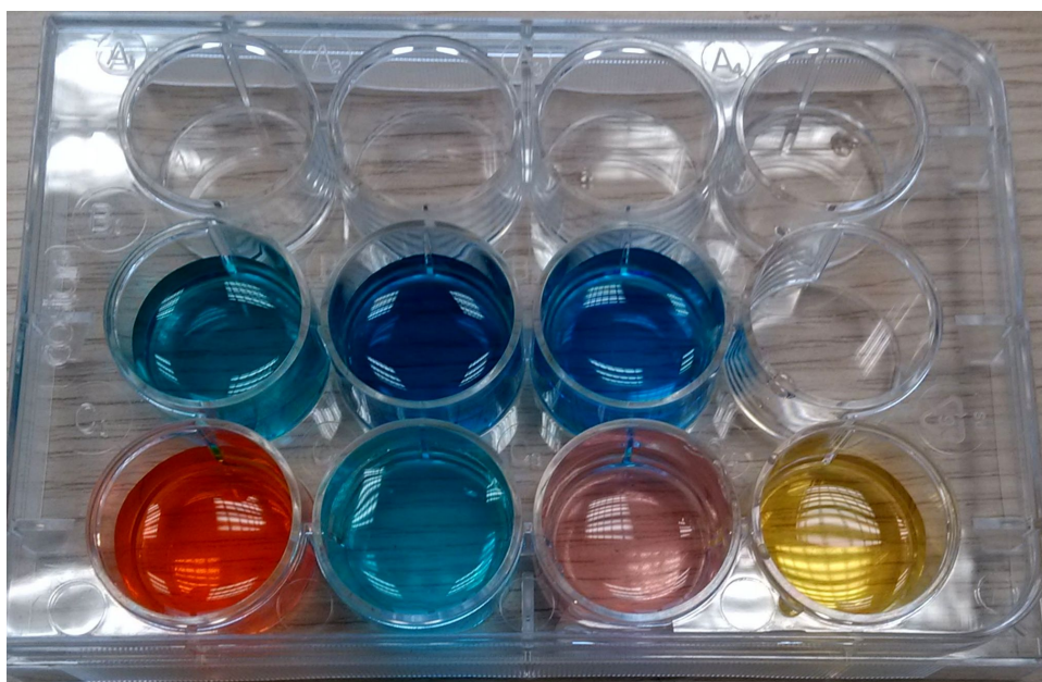
Figure 3.10: Second row (from left to right): Fast Green, Malachite Green, Methylene Blue. Third row (from left to right): Methyl Orange, CuSO_4 , CoCl_2 , Thymol
