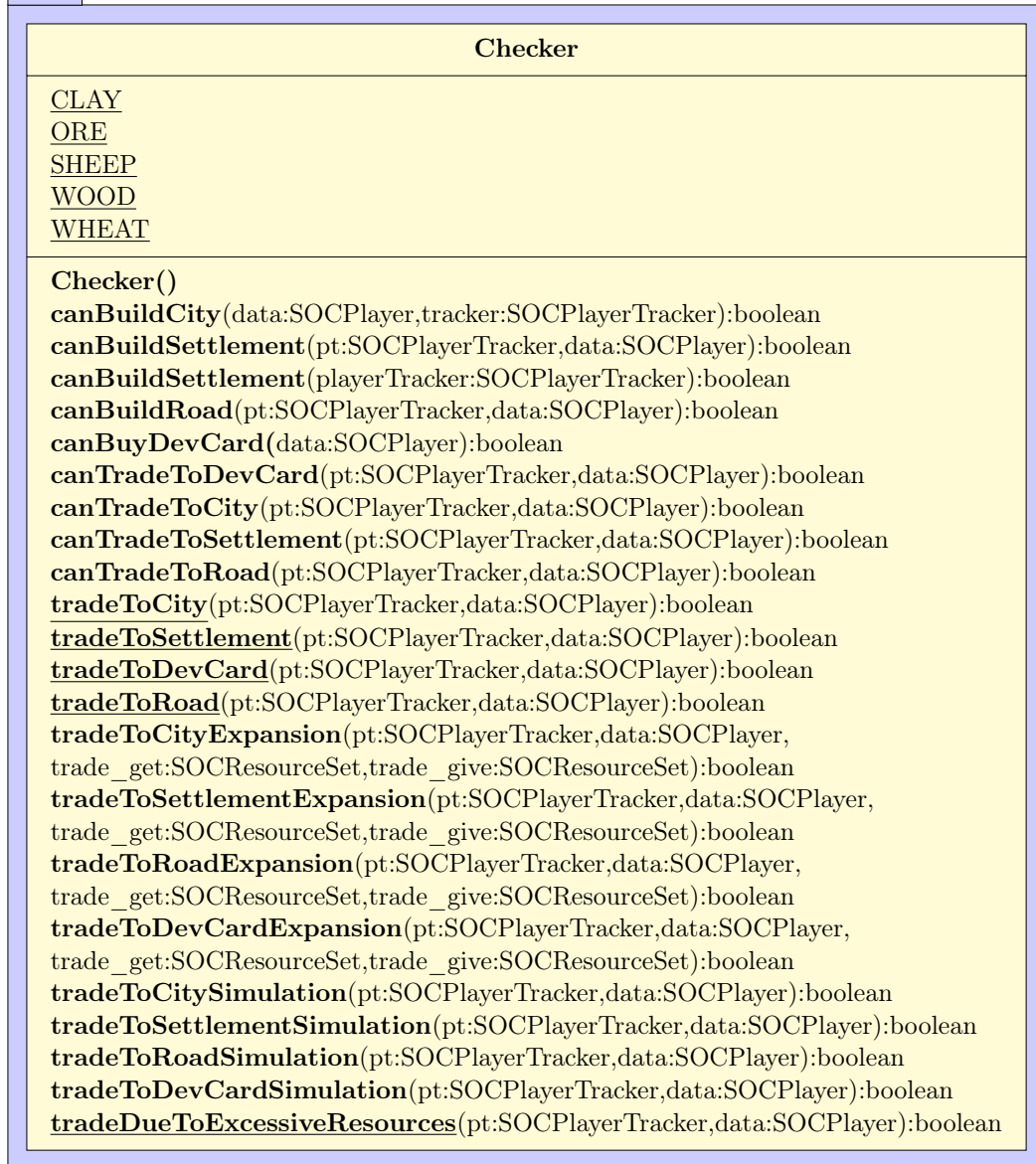
Figure 38: Class Diagram: Checker
