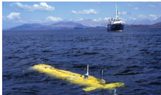
Figure 1.8: Autosub 1a Autonomous Underwater Vehicle on surface, ready for recovery. Picture by StifynTonna licensed under Creative Commons Attribution-Share Alike 3.0 Unported CC-BY-SA-3.0 license, via Wikimedia Commons.
