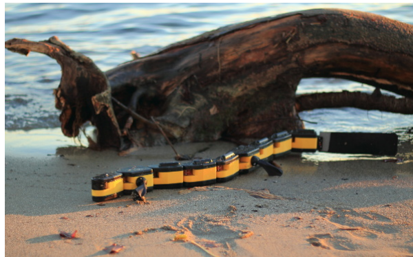
Figure 1.11: Salamander Robotica II , a biomimetic amphibious AUV. Picture by Kostas Karakasiliotis, Biorobotics Laboratory /Permission granted.
