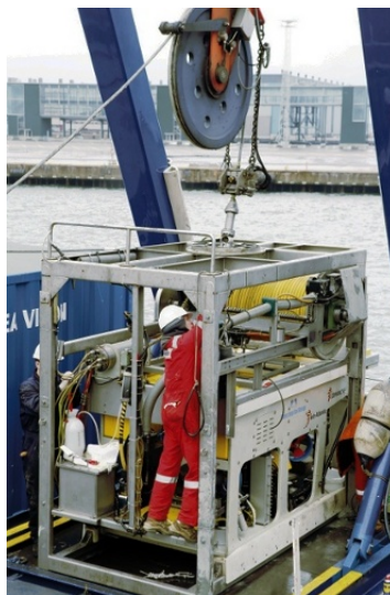
Figure 1.9: A Nord Stream ROV inside tether management system's garage , ready for launching. The garage is tethered to mothership's launch- recovery system. Picture by Nord Stream AG/Permission granted.
