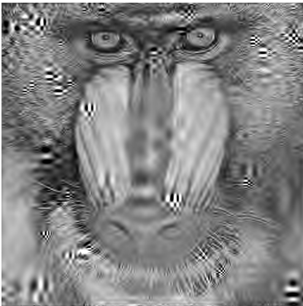
Illustration 25: 24: Baboon Joint decoding, BER=0.05 , 0.2\text{bpp} , LDPC 5/6
