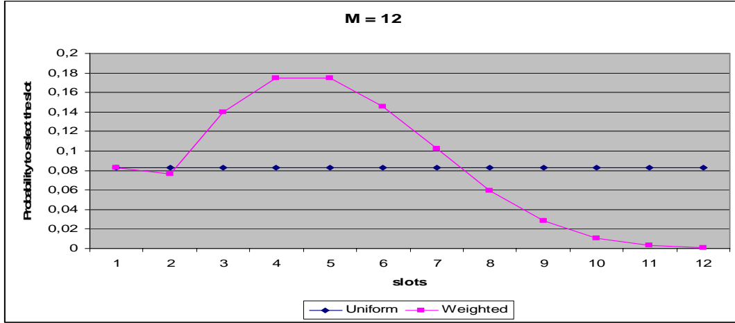
Figure 3. Comparison of the two slot selection schemes with 12 free slots in a channel frame.
