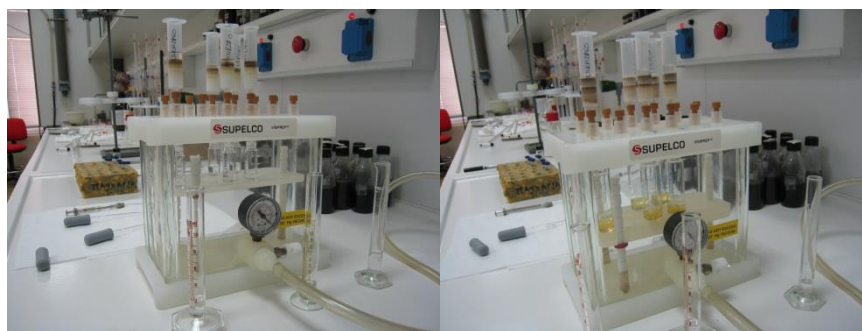
Figure 9: Solid Phase Extraction apparatus used for the fractionation of oil samples.
