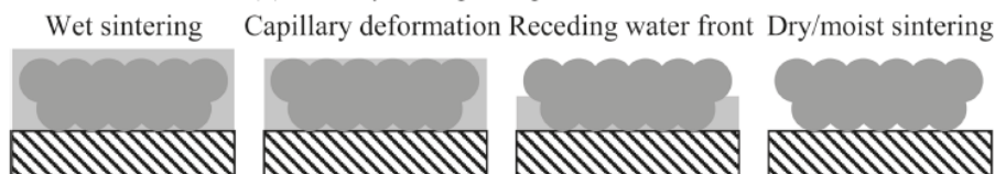
Figure 3.4: Condition of dispersion before stage II of particle deformation
