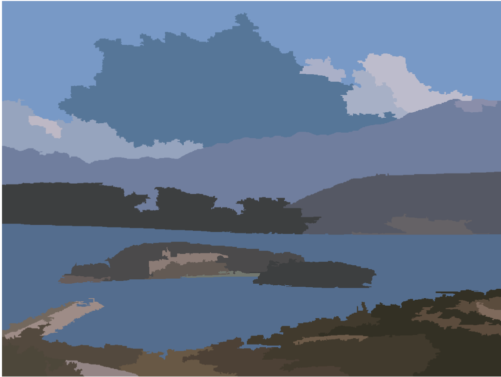
FIGURE 14: HIGH RESOLUTION IMAGE SEGMENTATION WITH MULTIPLE SKY REGIONS. INITIALLY, THE SEGMENTATION ALGORITHM DETECTS MANY REGIONS THAT BELONG TO THE SKY. THEY NEED TO BE MERGED TO PRODUCE A SINGLE SKY REGION.
