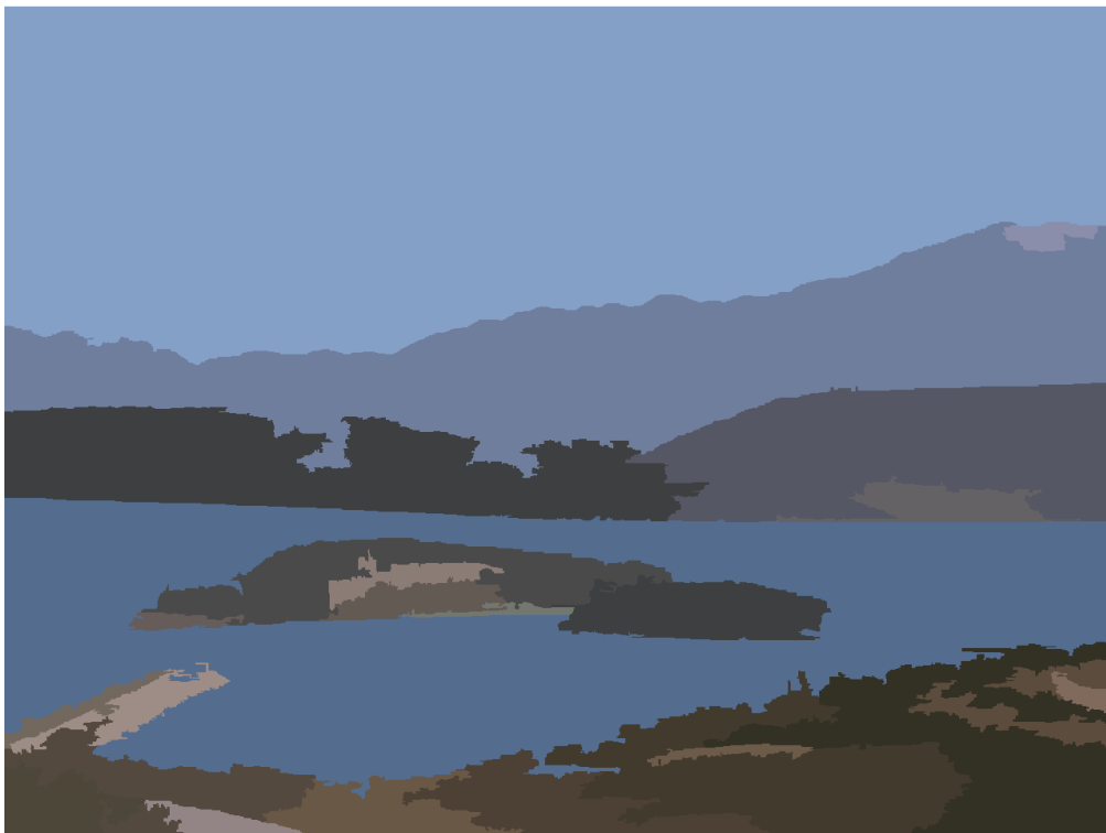
FIGURE 15: HIGH RESOLUTION IMAGE SEGMENTATION WITH THE SINGLE DETECTED SKY REGION. THE ALGORITHM HAS MERGED THE REGIONS THAT WERE NOT SMOOTH, CREATING A SINGLE REGION FOR THE SKY. THE SKYLINE CAN THEN BE EASILY EXTRACTED.
