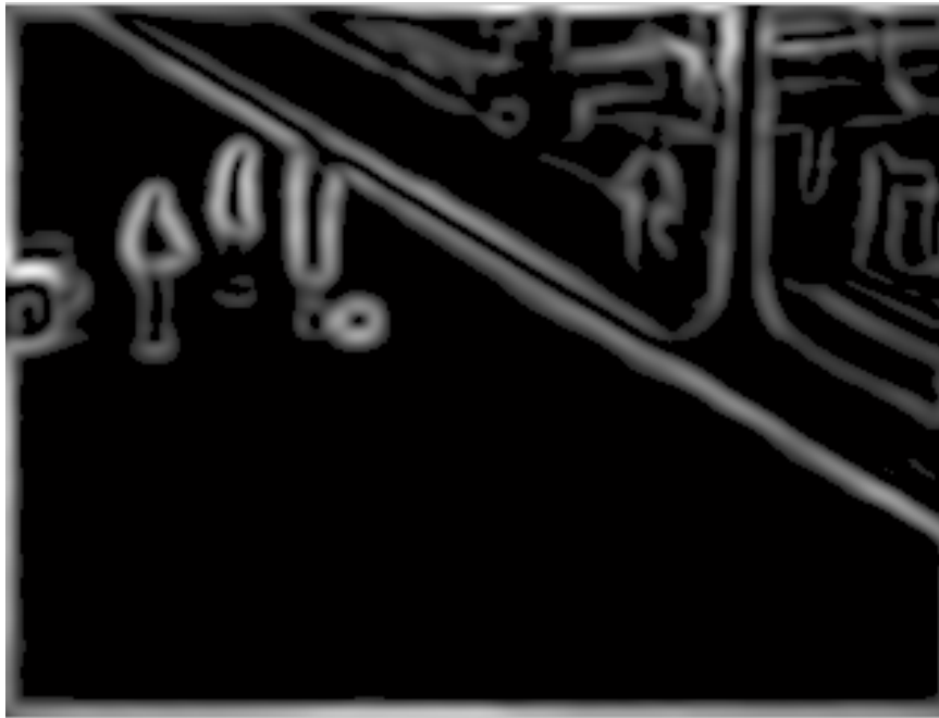
Figure 4.26: The edge image with scale factor \sigma = 3 ( T_g = 0.22 , P_{level} = 37.4 )
