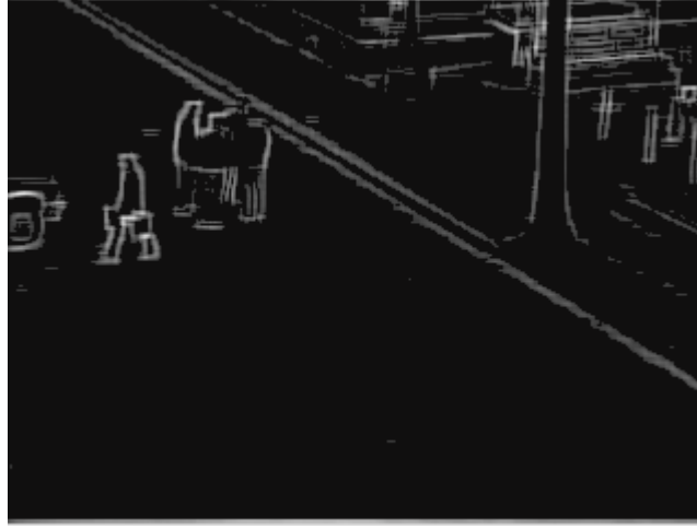
Figure 3.6: The proposed edge detector with \sigma = 2.0 ( T_g = 0.2 , P_{level} = 40.2 ).
