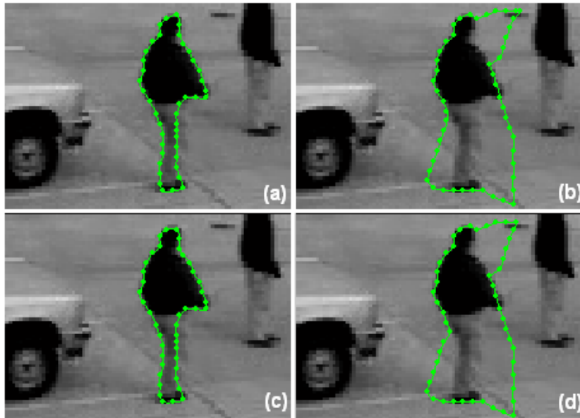
Figure 4.12: The resulting contours with (a,c) and without (b,d) the feedback mechanism, using the simplified (a,b) or the compound-parameter (c,d) convergence criterion.
