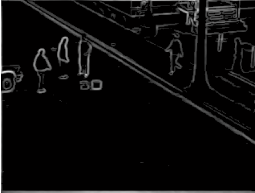
Figure 4.25: The edge image with scale factor \sigma = 1 ( T_g = 0.22 , P_{level} = 38.28 )
