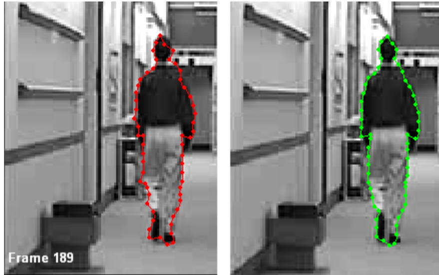
Figure 4.36: Tracking of object using the “scale-space” model (video B).
