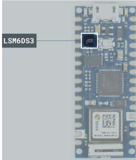
Figure 19: Location of the on-board IMU (LSM6DS3) on the Arduino Nano 33 IoT used to sense lean angle and angular rate. USB connector at the top for orientation. [24] [25]
