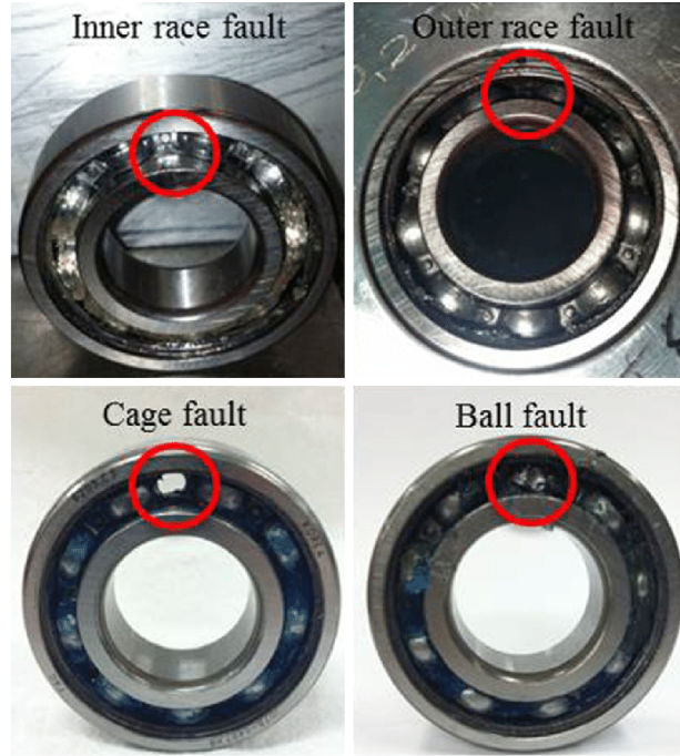
Figure 2.21: Bearing type faults [60].
