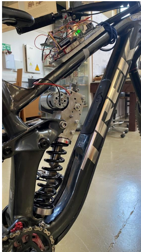
Figure 32: The bicycle with the absorber installed and the electrical circuit attached on it
