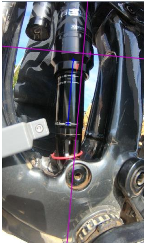
Figure 11: Set-up process of the axle and calibration stick in Tracker software.
