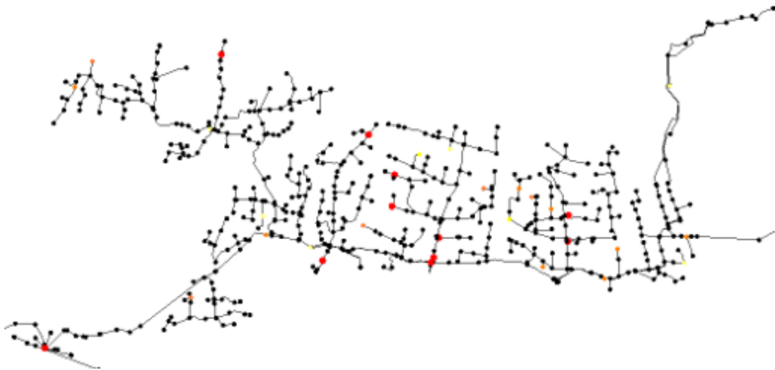
Figure 23: Some potential leaks at 3 hours
