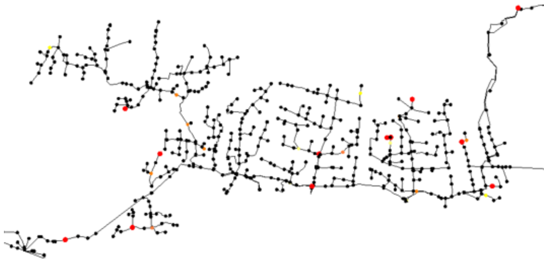
Figure 24: Some potential leaks at 28 hours
