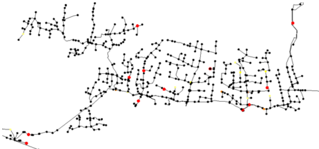
Figure 25: Some potential leaks at 53 hours
