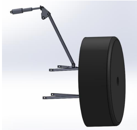
Fig 19 : Cad Model of the Front Suspension
