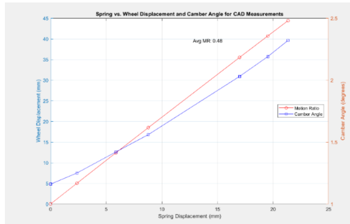
Fig 40 :Motion Ratio and Camber gain
