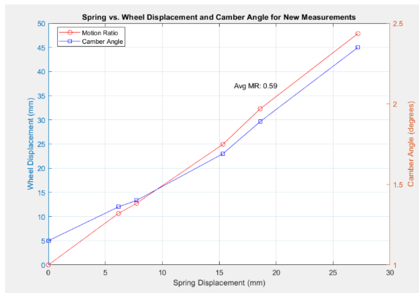
Fig 44: Motion Ratio and Camber gain
