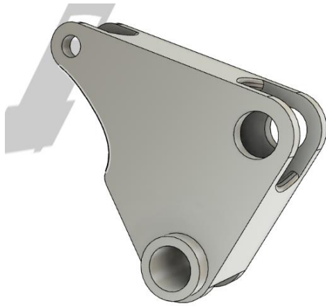
Fig 14 : Detailed view of the Rocker Arm
