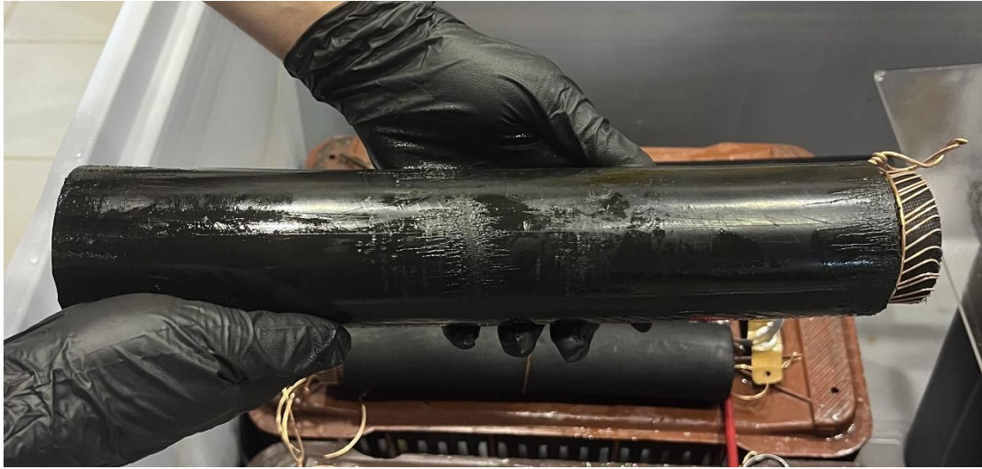
Figure 40. Cable after surface discharge.
