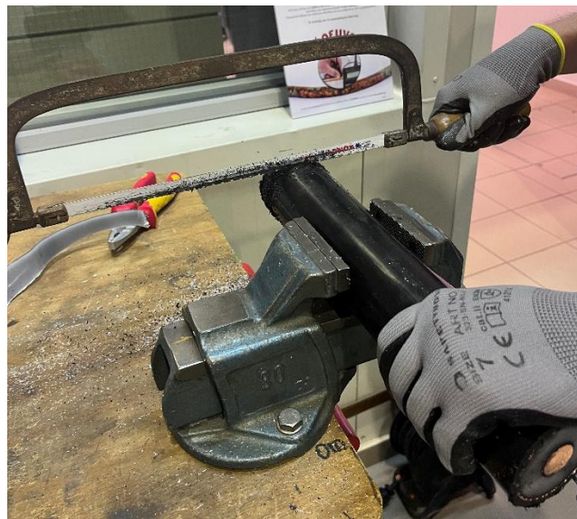
Figure 28. Saw and slicing procedure.
