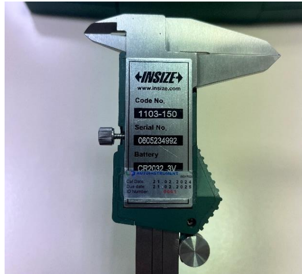
Figure 31. Vernier caliper for thickness measurement.
