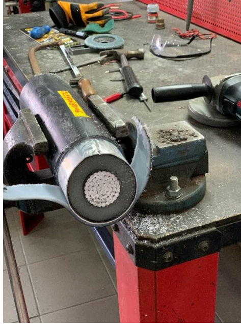
Figure 46. 150kV specimen with jacket ring removed.
