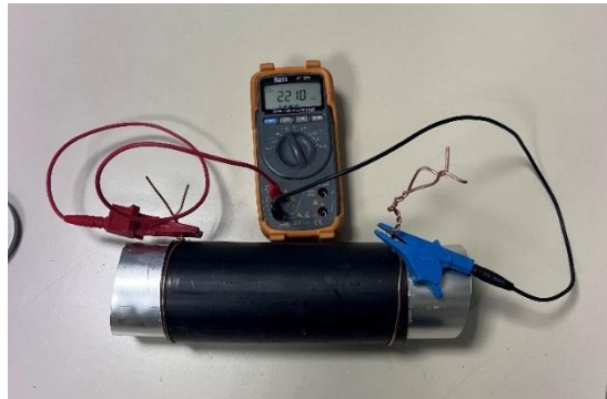
Figure 50. Resistance measurement for 150kV rated cable.
