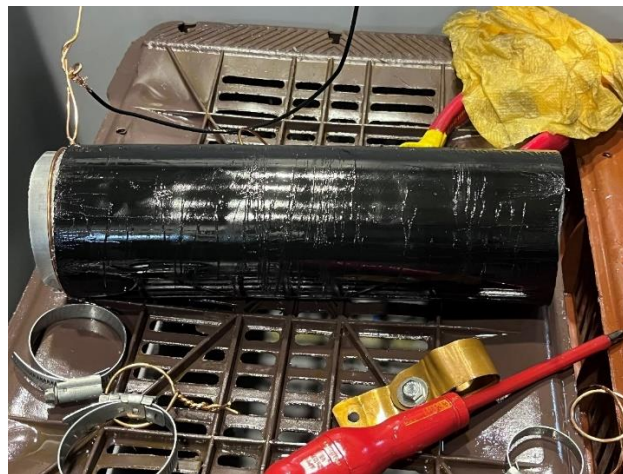
Figure 51. Burned jacket of specimen zero.
