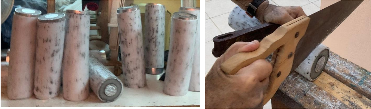
Figure 52. Removal of semiconductive layer and specimen preparation.
