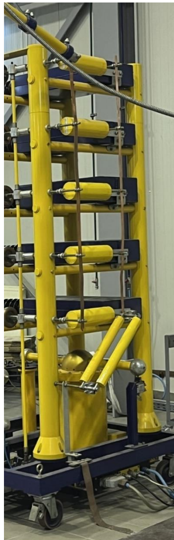
Figure 22. Tail and front resistors repositioned.
