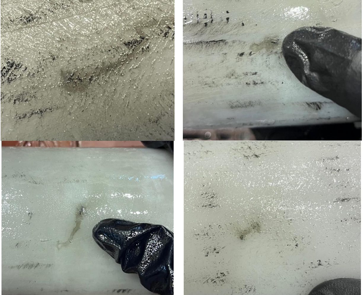
Figure 54. Examples of jacket insulation failures.
