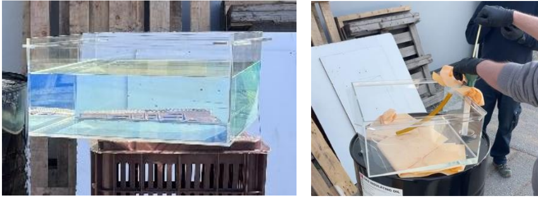
Figure 8. Oil filling with manual pump.
