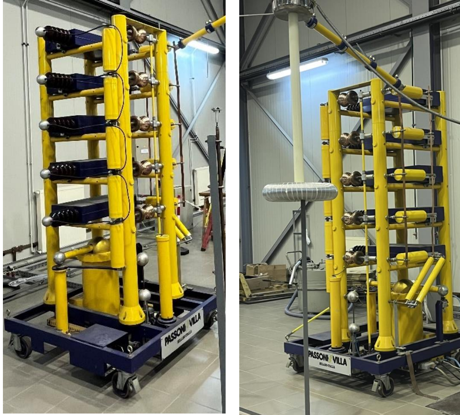
Figure 24. Fully assembled single-stage voltage impulse generator.
