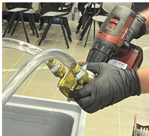
Figure 10. New oil filling process.
