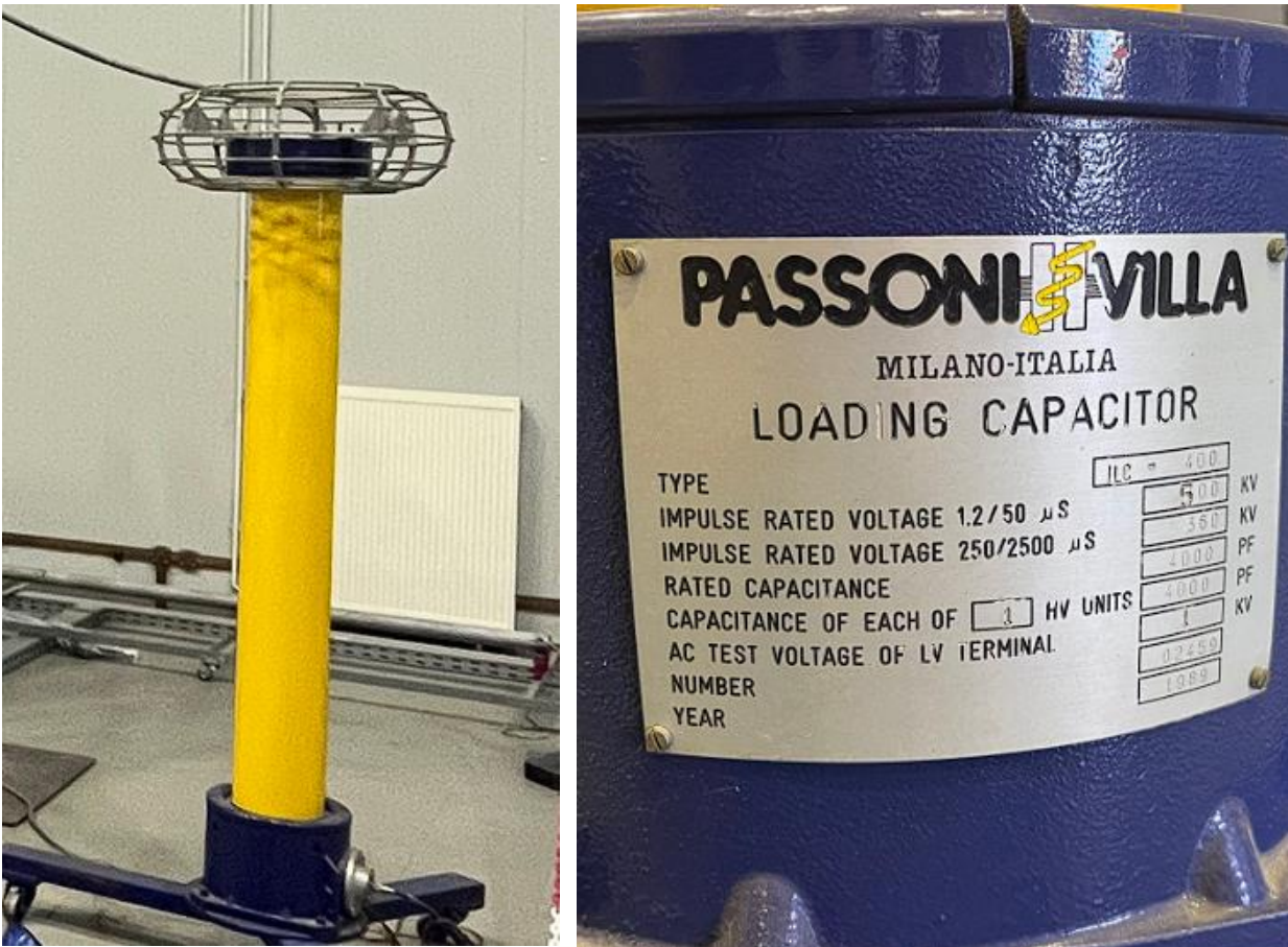
Figure 33: Impulse Voltage Divider (left) and its technical specifications (right).
