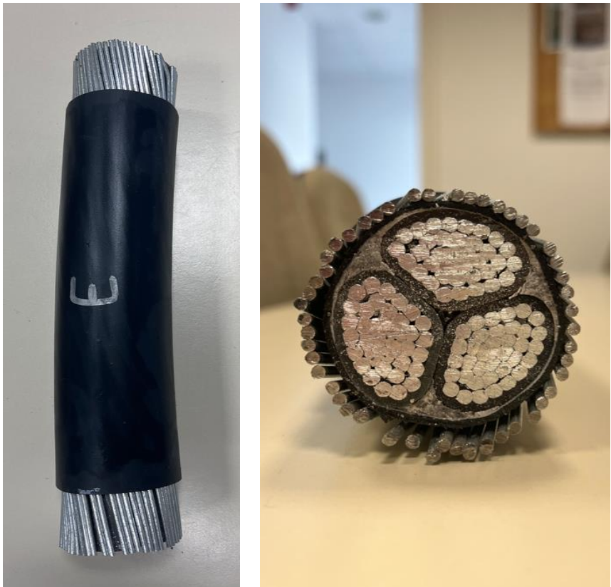
Figure 14:Photographs of the actual Cable E sample used in the experimental setup: (left) side view of the cable segment with partially stripped outer sheath, and (right) cross-sectional view showing the conductor bundle, insulation, and exposed screen layers.
