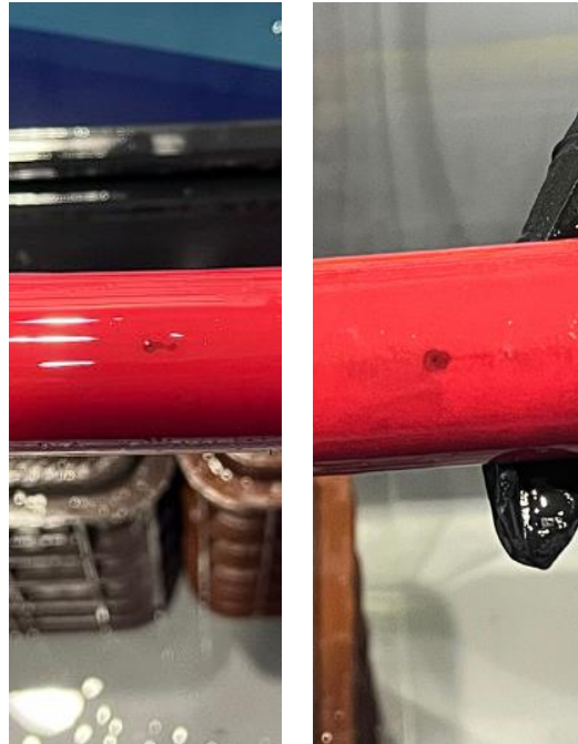
Figure 46: Visible breakdown jacket markings in Cable C.
