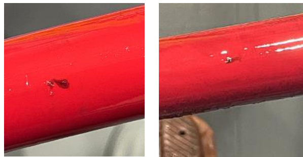
Figure 49: Visible breakdown jacket markings in Cable D.
