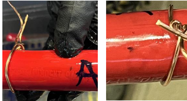
Figure 40: Visible breakdown markings and localized discharge path.
