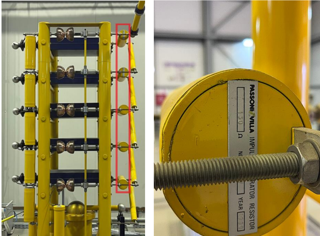
Figure 26: Tail resistors and their highlighted position in the generator (left) and rating label (right).
