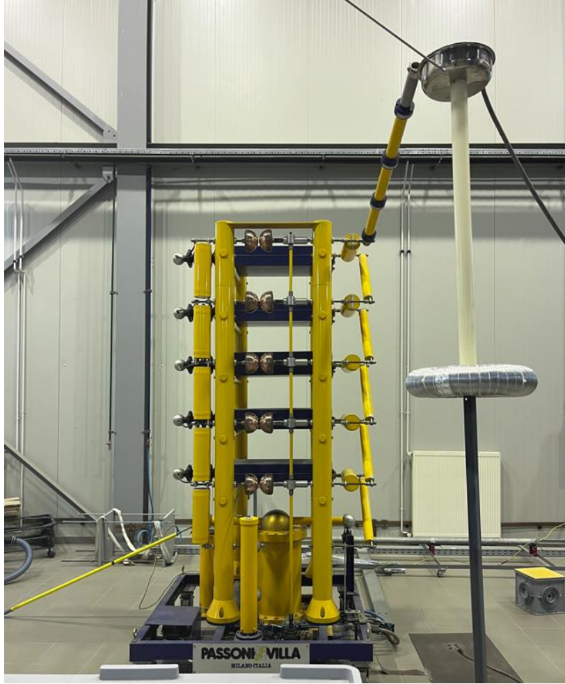
Figure 20: Front view of the five-stage Marx generator.
