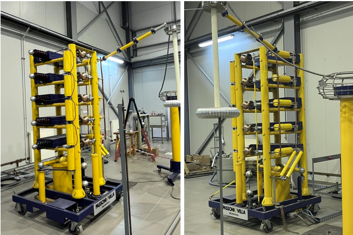
Figure 32: Left and right view of the Marx generator parallelized configuration.
