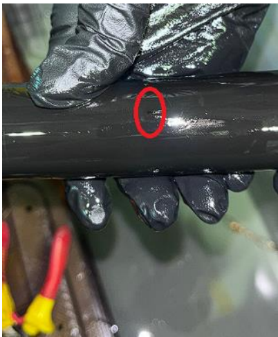
Figure 43: Visible breakdown jacket marking in Cable B.
