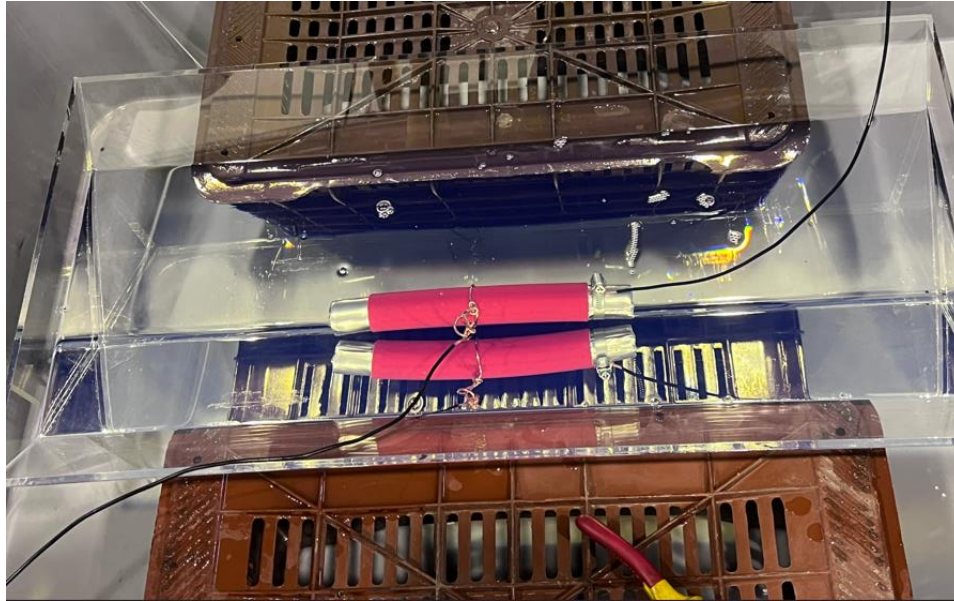
Figure 16: Overview of the second experimental oil tank arrangement with cable sample.
