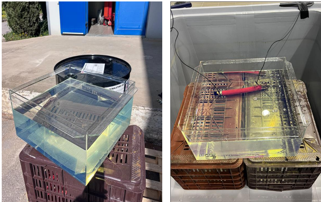
Figure 15: Overview of the first dielectric oil tank (left) and experimental arrangement with cable sample (right).
