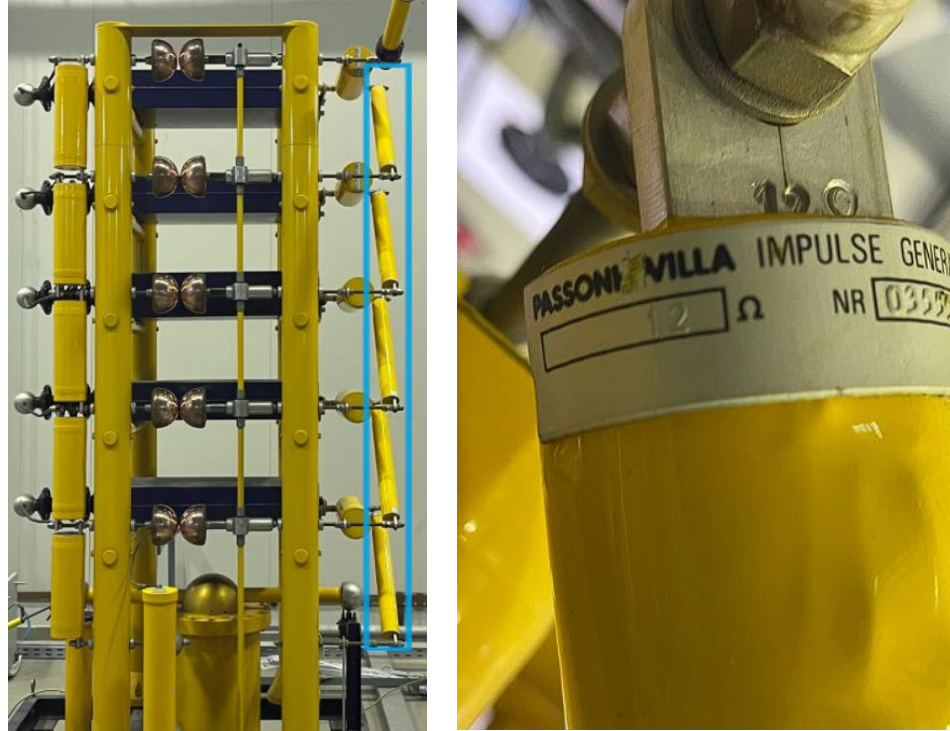
Figure 25: Front resistors and their highlighted position in the generator (left) and rating label (right).
