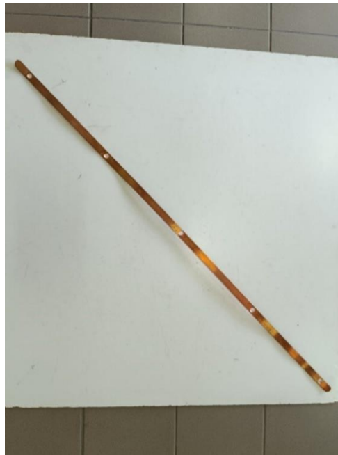
Figure 30: Copper bus bar used for parallelizing capacitors.
