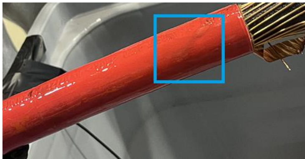
Figure 42: Surface discharge trace on the PVC jacket of Cable A.
