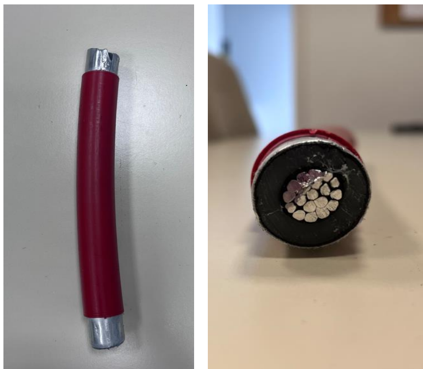
Figure 12: Photographs of the actual Cable D sample used in the experimental setup: (left) side view of the cable segment with partially stripped outer sheath, and (right) cross-sectional view showing the conductor bundle, insulation, and exposed screen layers.
