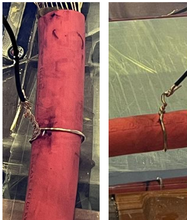
Figure 39: Cable A samples immediately after an electrical breakdown.
