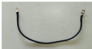
Figure 31: Short insulated conductor used for connecting charging resistors ( R_c ) to the DC source.
