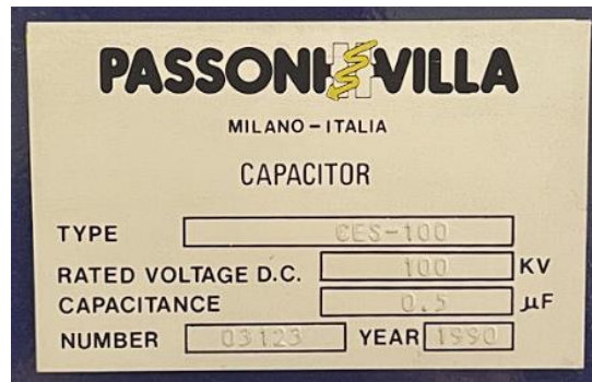
Figure 22: Nameplate of the Marx generator capacitor.
