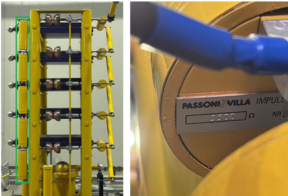
Figure 23: Charging resistors and their highlighted position in the generator (left) and rating label (right).
