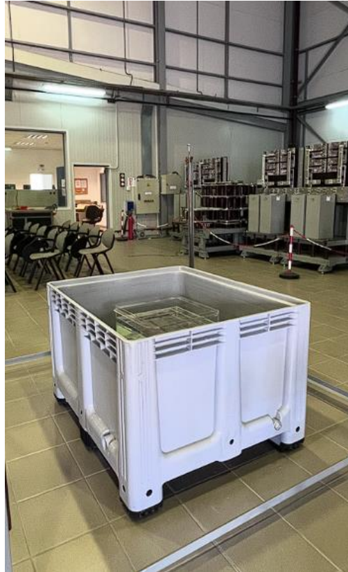
Figure 19: Safety containment box that houses the test tanks.
