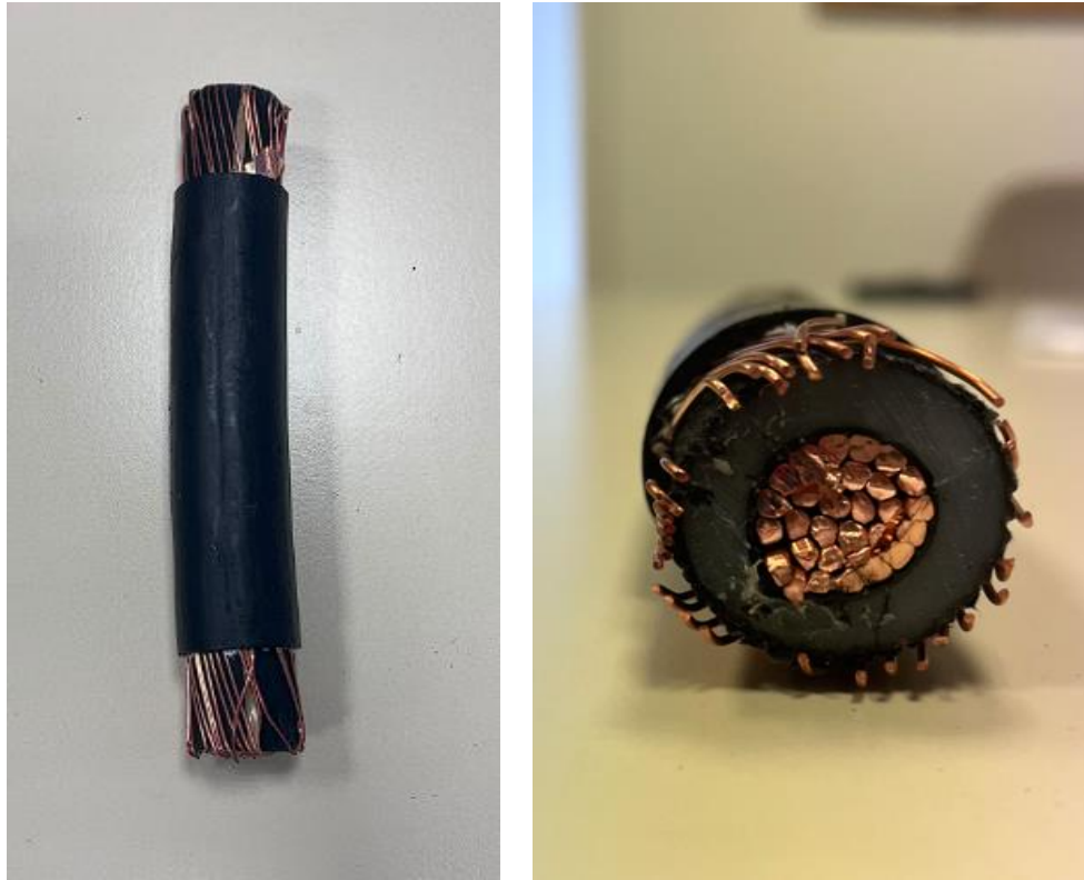
Figure 8: Photographs of the actual Cable B sample used in the experimental setup: (left) side view of the cable segment with partially stripped outer sheath, and (right) cross-sectional view showing the conductor bundle, insulation, and exposed screen layers.
