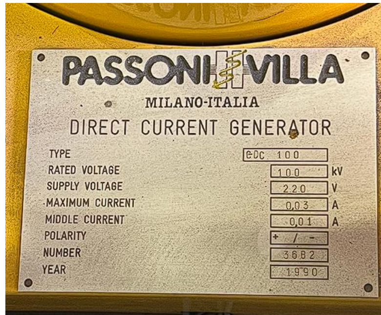
Figure 21: Nameplate of the Direct Current Generator.
