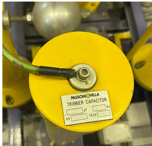
Figure 24: Trigger capacitor installed at the Marx generator.
