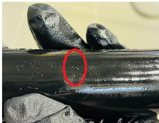
Figure 51: Visible breakdown jacket marking in Cable E.
