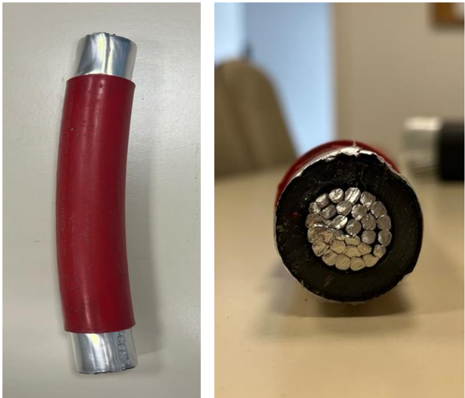
Figure 10: Photographs of the actual Cable C sample used in the experimental setup: (left) side view of the cable segment with partially stripped outer sheath, and (right) cross-sectional view showing the conductor bundle, insulation, and exposed screen layers.
