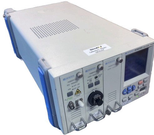
Figure 3.2 : Photography of Yokogawa Ando with a AQ8201-13 module.
