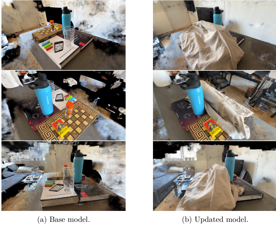
Figure 4.16: From the above figure, we observe that the model is once again able to robustly reconstruct the updated scene, successfully integrating the added shirt despite it obscuring a significant portion of the original setup. Importantly, the consistency and integrity of the remaining scene elements are preserved, demonstrating the model’s resilience in handling occlusions without degrading the quality of previously learned content. The total training time to reach the final model was 36 minutes: 28 minutes for the base (a) model and 8 minutes for the updated (b) model.
