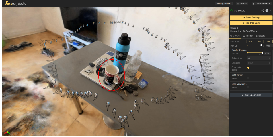
Figure 3.8: Nerfstudio viewer result, showing that new object (mug) was successfully learned by the model and added to the scene.
