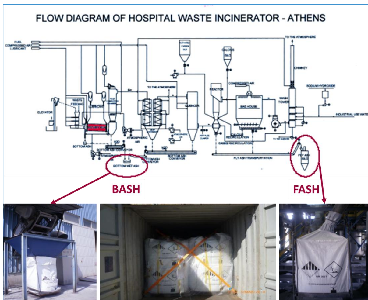
Image 2: The flow diagram of the HMWIP operated by “APOTEFROTIRAS S.A.”. The bottom (BASH) and fly (FASH) ashes collected in appropriate bags and their final disposal storage place in the plant (Kougemitrou, 2008; Kougemitrou et al., 2011; HMWIP internal report)
