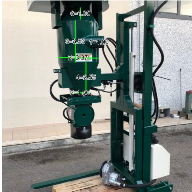
Figure 26: Pixel ratio of cyclone's parameters relative to the hose's inlet flange. [Source for image: "crfcostruzioni.it", source for image measurements: " https://eleif.net/photomeasure "]
