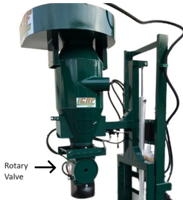
Figure 60: Rotary valve component, mounted at the bottom of the cyclone. The continuously rotating vanes inside the rotary valve casing unload the olive fruits at a constant rate. [Source for image: " crfcostruzioni.it "]
