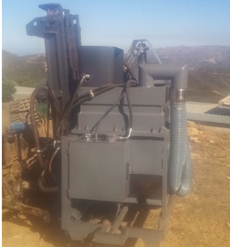
Figure 50: Aspirator device with rectangular box. The hydraulic system for the impeller's rotation is also visible.
