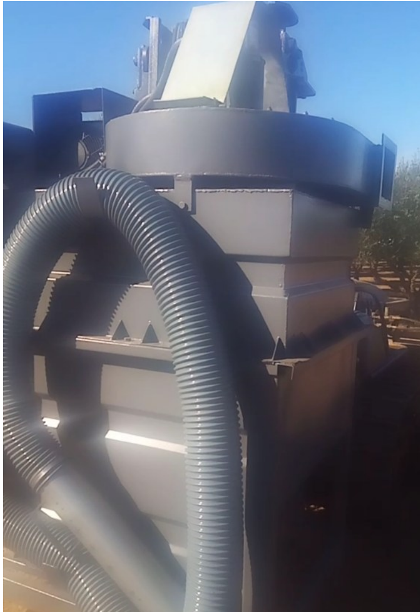
Figure 59: Box aspirator device completed assembly.
