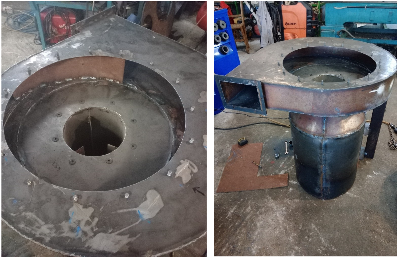
Figure 32: Result of manufacturing process of the impeller's casing.
