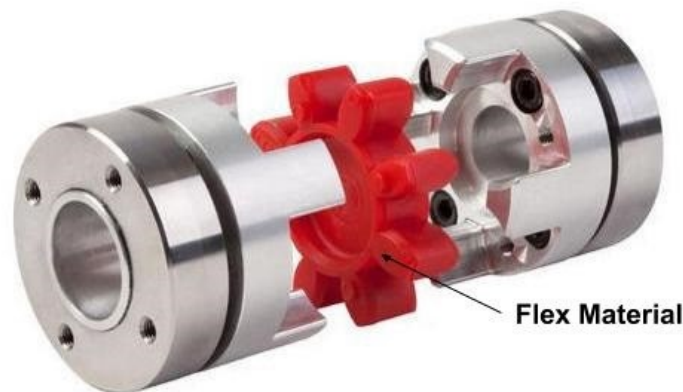
Figure 36: Jaw-type mechanical coupler. It is used for damping torsional vibrations between the connected shafts. [Source: https://www.smlease.com/entries/mechanism/what-is-mechanical-coupling-types-applications ]
