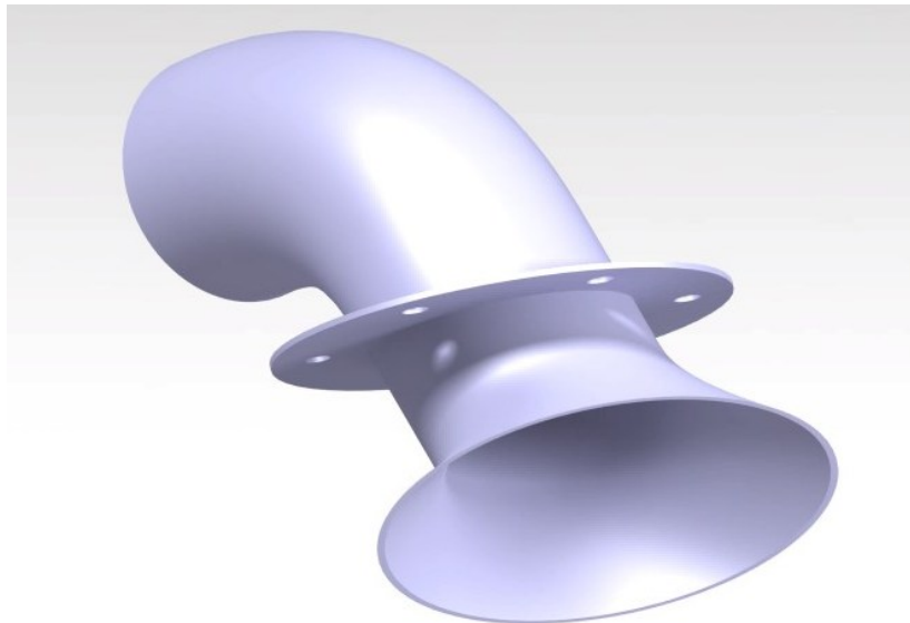
Figure 47: Hose's inlet flange with a diffuser
