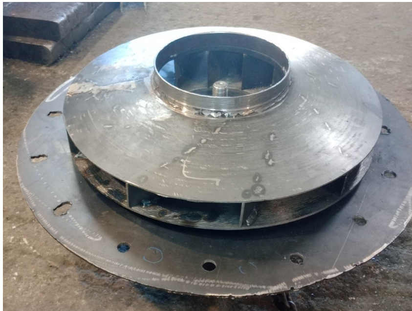
Figure 38: The blower is mounted to the shaft. Also, the shaft is supported to the bottom flange of the casing.
