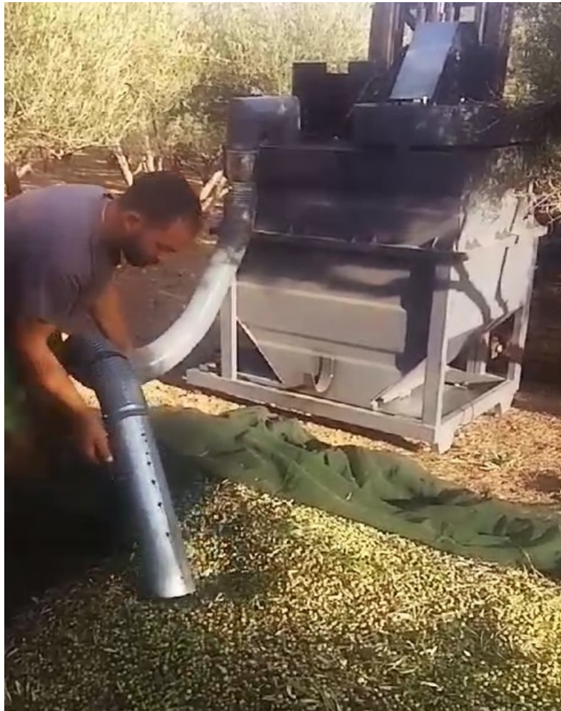
Figure 52: Aspirator device operating on the field. The hose length was shortened to minimize curve formation in the hose's path.
