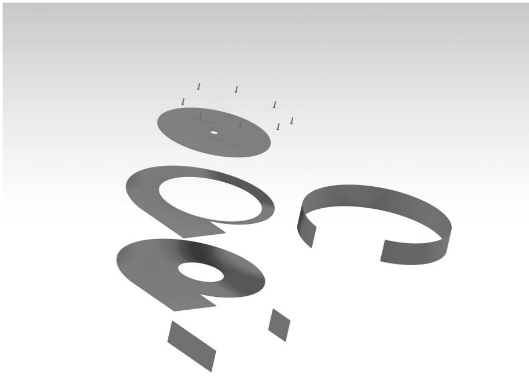
Figure 31: Exploded view of the impeller's casing. In this view all the individual flanges can be seen before welding together.
