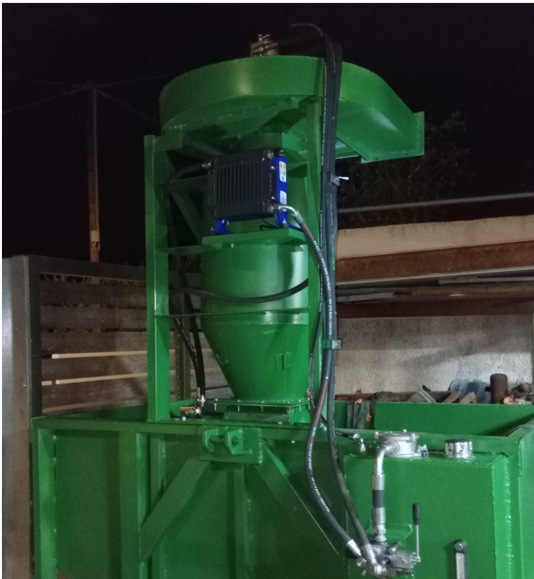
Figure 27: Aspirator device with cyclone. The assembly of the device includes the hydraulic system for the impeller's rotation.
