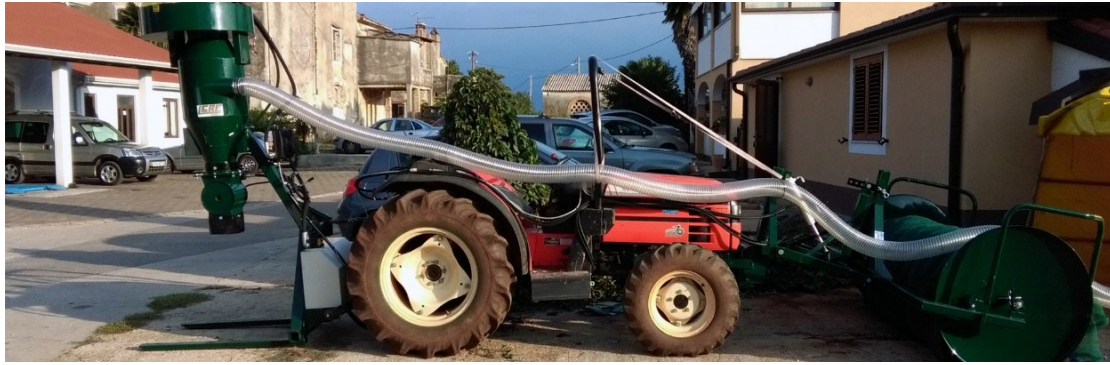
Figure 19: Aspirator device with cyclone. [Source: crfcostruzioni.it ]
