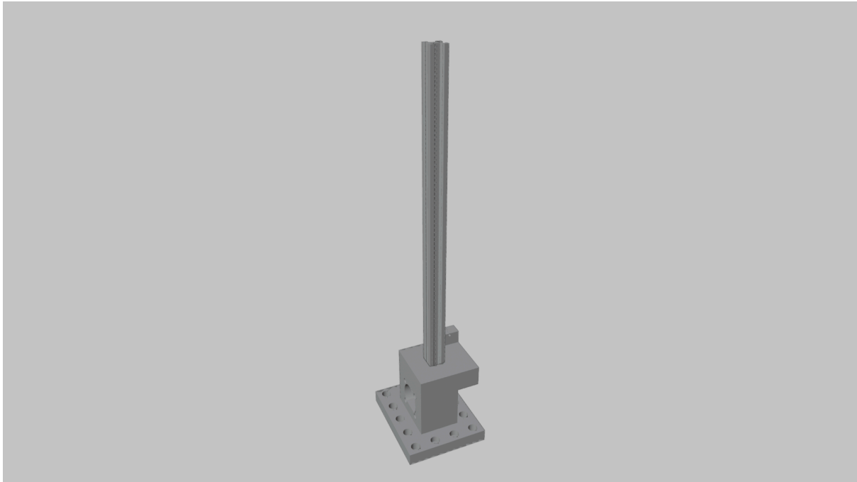
Figure 14: Vertical axis and motor mount.
