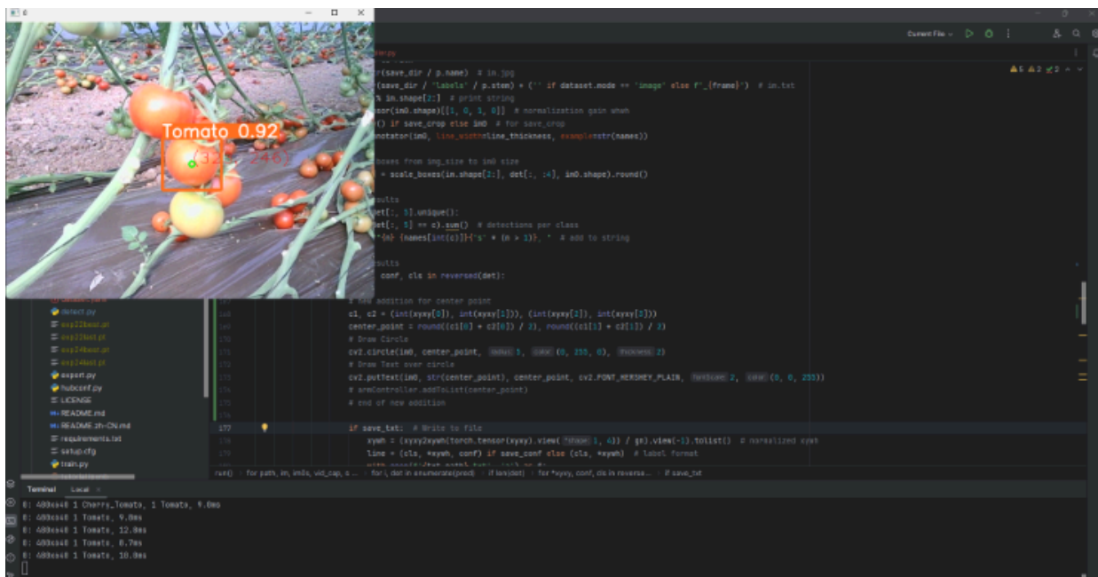
Figure 34: Tomato detection with bounding box.
