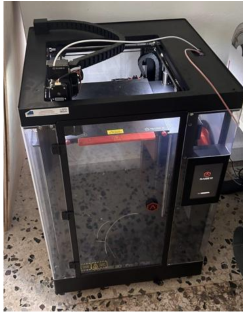
Figure 22 : The Raise3D Pro2 Plus 3D printer that was used to print the parts.
