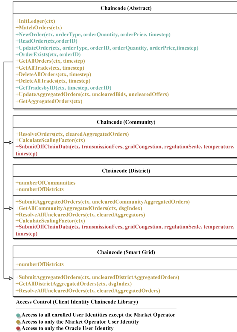
Figure 4.4 – UML Schema presenting the contractual extension of Chaincodes for Community, District, and Smart Grid contracts.
