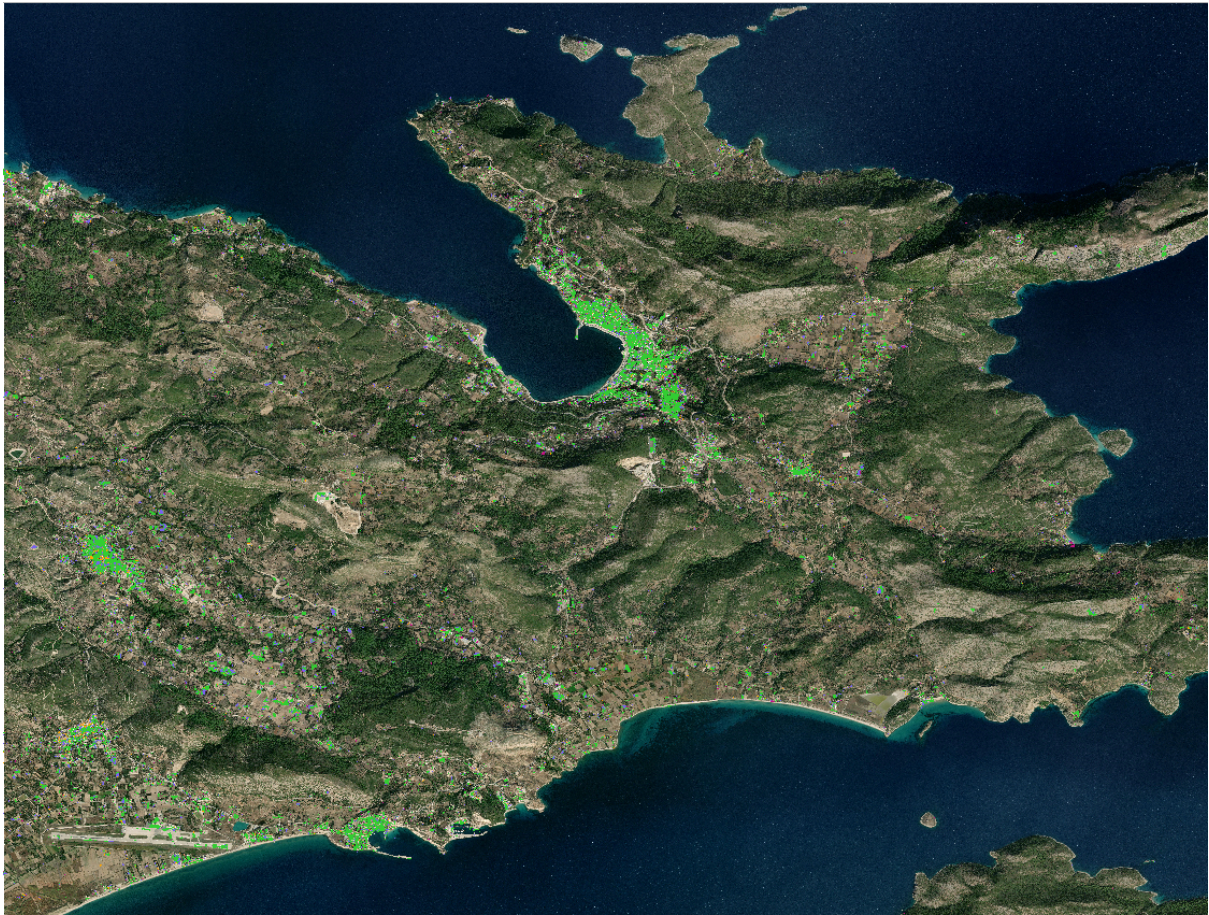
Figure 5.13. Building damage map of Samos, Greece generated by the proposed pipeline.
