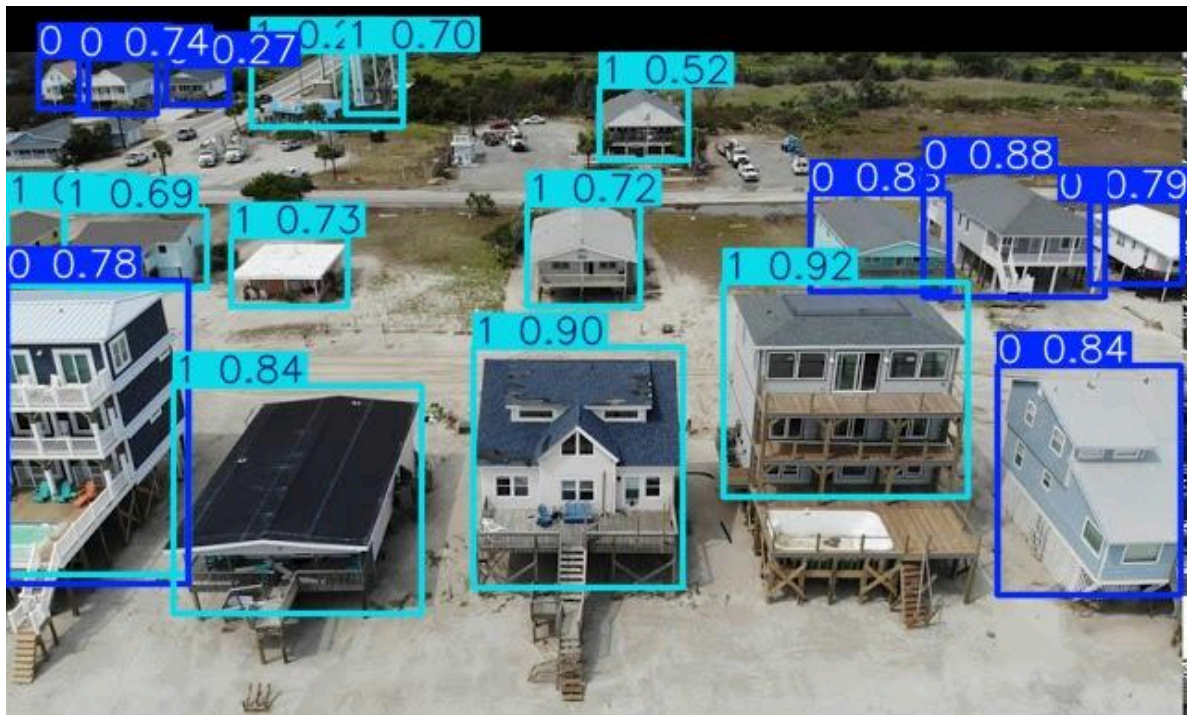
Figure 5.23.c. Building damage bounding boxes on imagery from the United States by the proposed pipeline.
