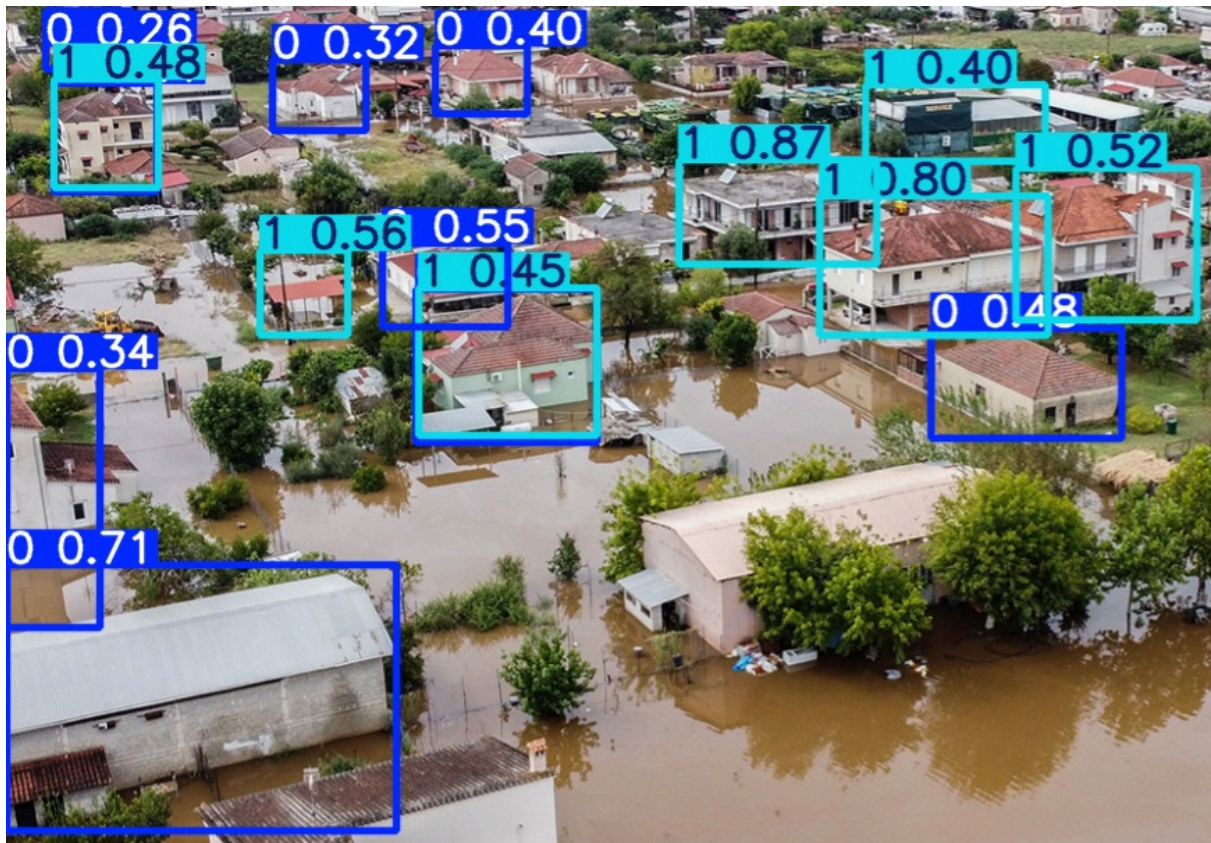
Figure 5.24.c. Building damage bounding boxes on imagery from Thessaly, Greece by the proposed pipeline.
