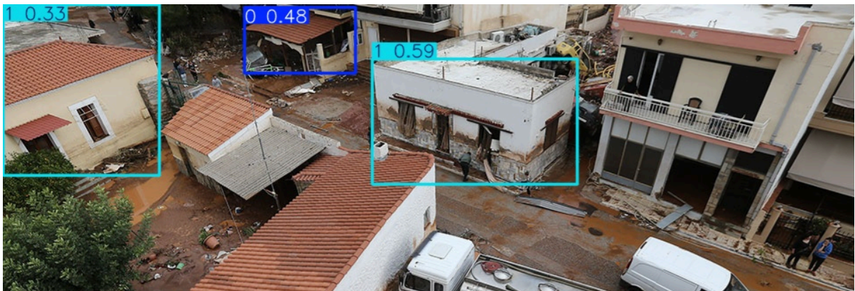
Figure 5.24.b. Building damage bounding boxes on imagery from Thessaly, Greece by the proposed pipeline.
