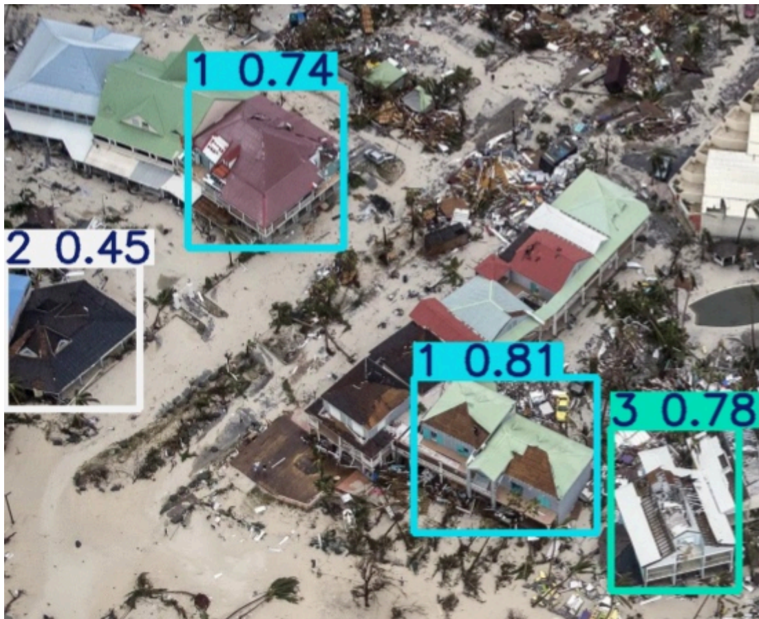
Figure 5.23.f. Building damage bounding boxes on imagery from the United States by the proposed pipeline.
