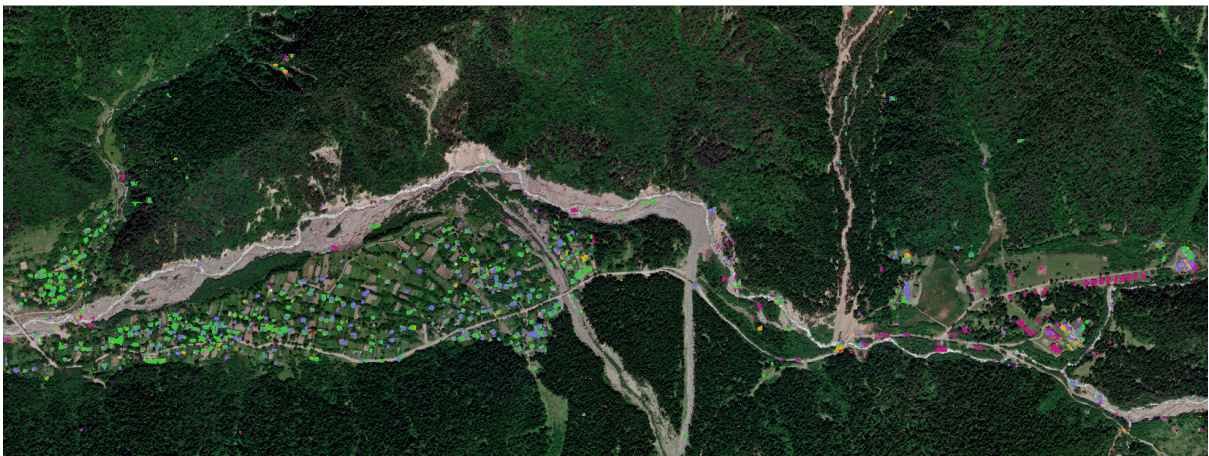
Figure 5.19. Building damage map of Shovi, Georgia generated by the proposed pipeline. Area of the landslide is highlighted on the right side.
