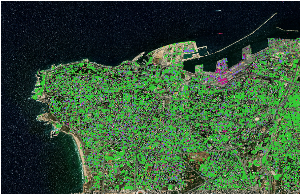
Figure 5.7. Building damage map of Beirut, Lebanon generated by the proposed pipeline. Area of explosion is highlighted in the top right corner.
