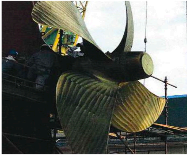
Picture 8-Propeller after cleaning-polishing
