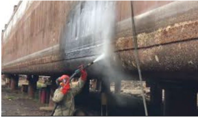
Picture 6-Sandblasting during dry dock
