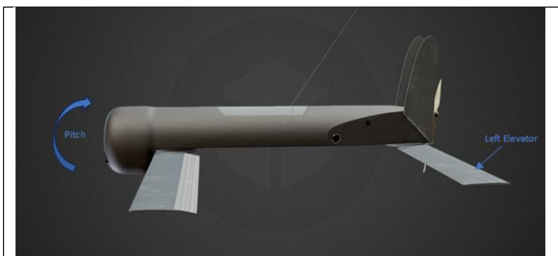
Figure 52: Elevators and pitch
