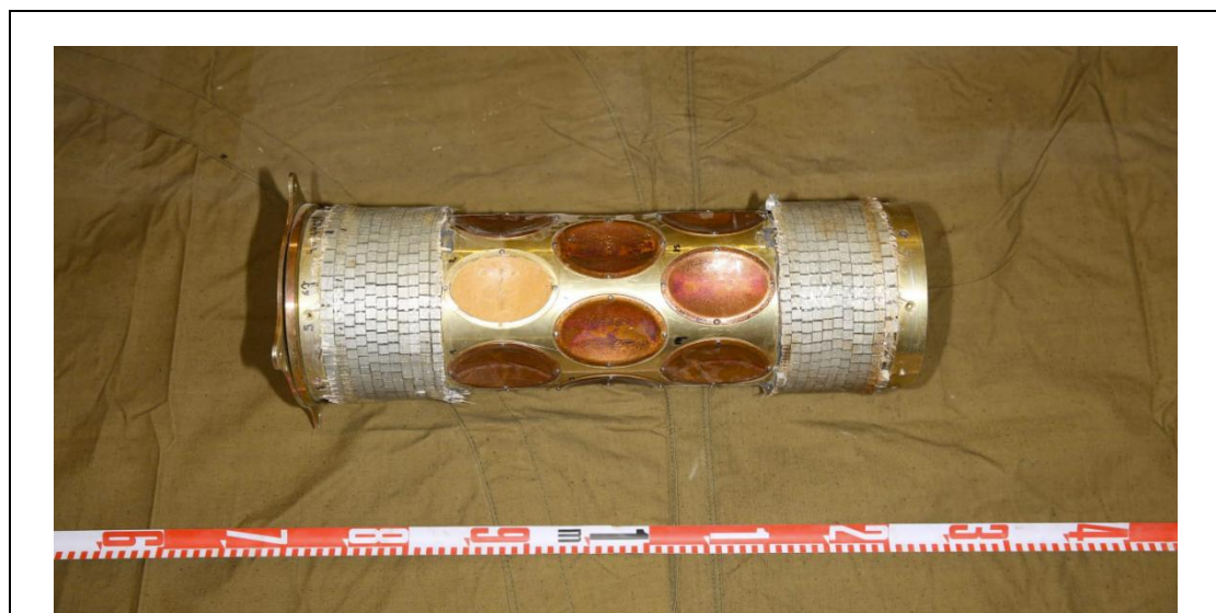
Figure 77: Warhead for the Shahed – 131 kamikaze drone (ISIS, 2024)
