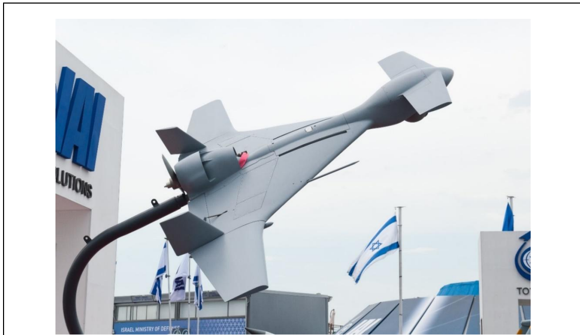
Figure 41: Canard configuration (Wikipedia, 2020)
