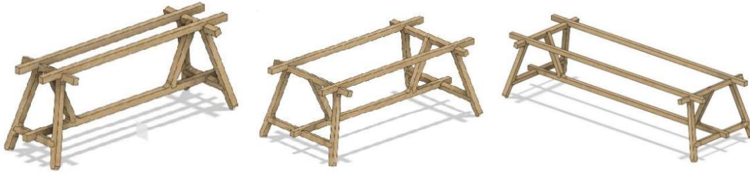
Figure 8 Example of multiple instances of a digital twin CAD model
