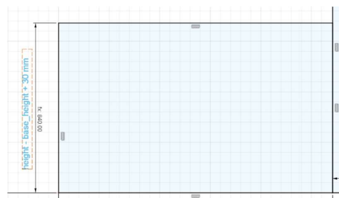
Figure 42 Equations for creating envelopes for door panels
