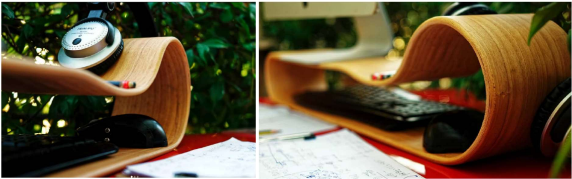
Figure 1 Bent lamination monitor stand, made in August 2019. Entry for international competition “Rockler Bent Wood Challenge”. Multiple veneer layers of differing length laminated using mold techniques to form a continuous loop of wood grain used to keep computer accessories in order. Designed and manufactured by Zygoulis Nikolas
