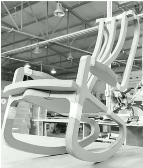
Figure 3 Prototype rocking chair. made in Feb 2021. One-half scale. Nested MDF parts machined using basic techniques to produce intricate joinery. Designed and manufactured by Zygoulis Nikolas
