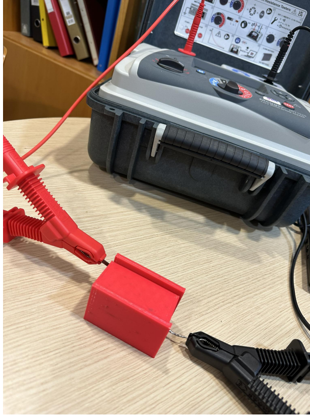
Figure 3.16: R_{cc} measurement procedure.
