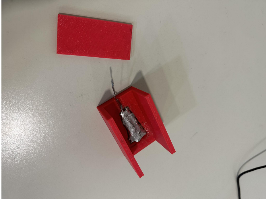
Figure 3.15: Custom pastic casing with conductive floor. As it can be seen a metal wire is protruding from the conductive floor to make the connection with the testing equipment possible.
