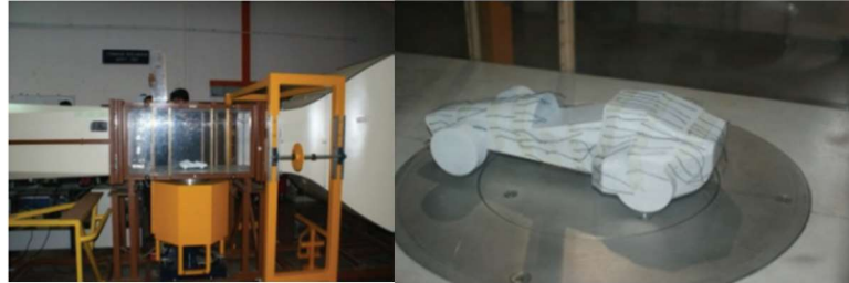
Figure 21: The wind tunnel and the 1/10 scale model used (Hetawal, et al., 2014).
