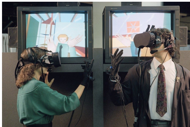
Figure 2.4: A demonstration of the EyePhone system, which uses special goggles, and a DataGlove, allowing users to see and manipulate objects around in a computer created environment [3].
