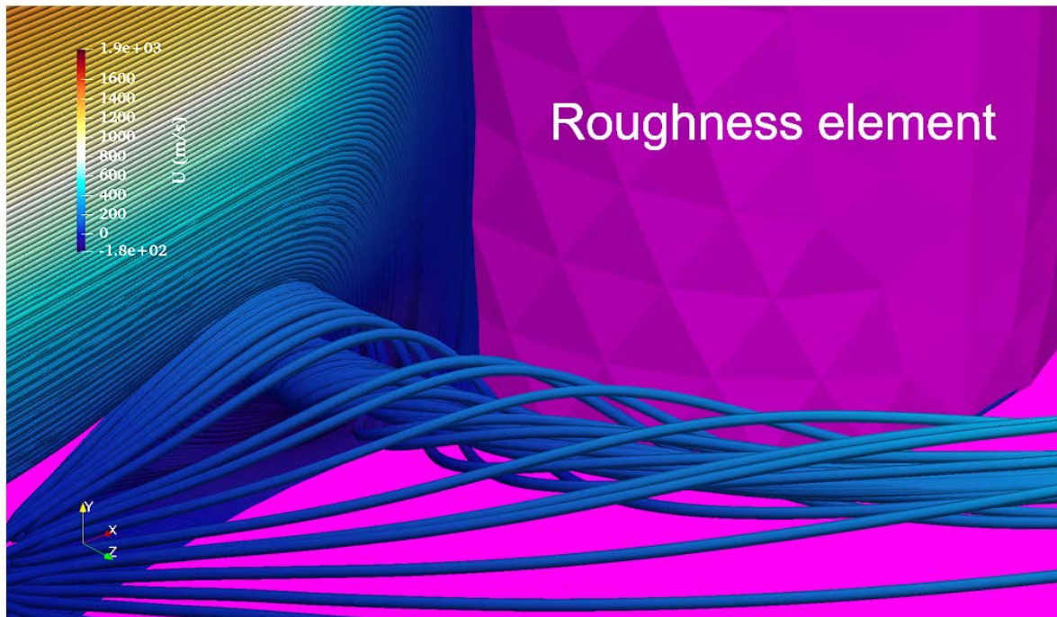
Figure 3.90. Vortex core streamlines at the base of the roughness element.
