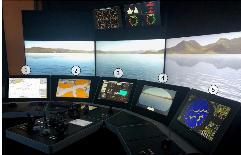
Figure 2.18: A simulator for testing and assessing human supervised autonomous ship navigation
