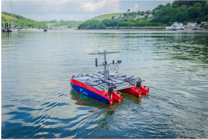
Figure 2.2: USV to research water pollution
