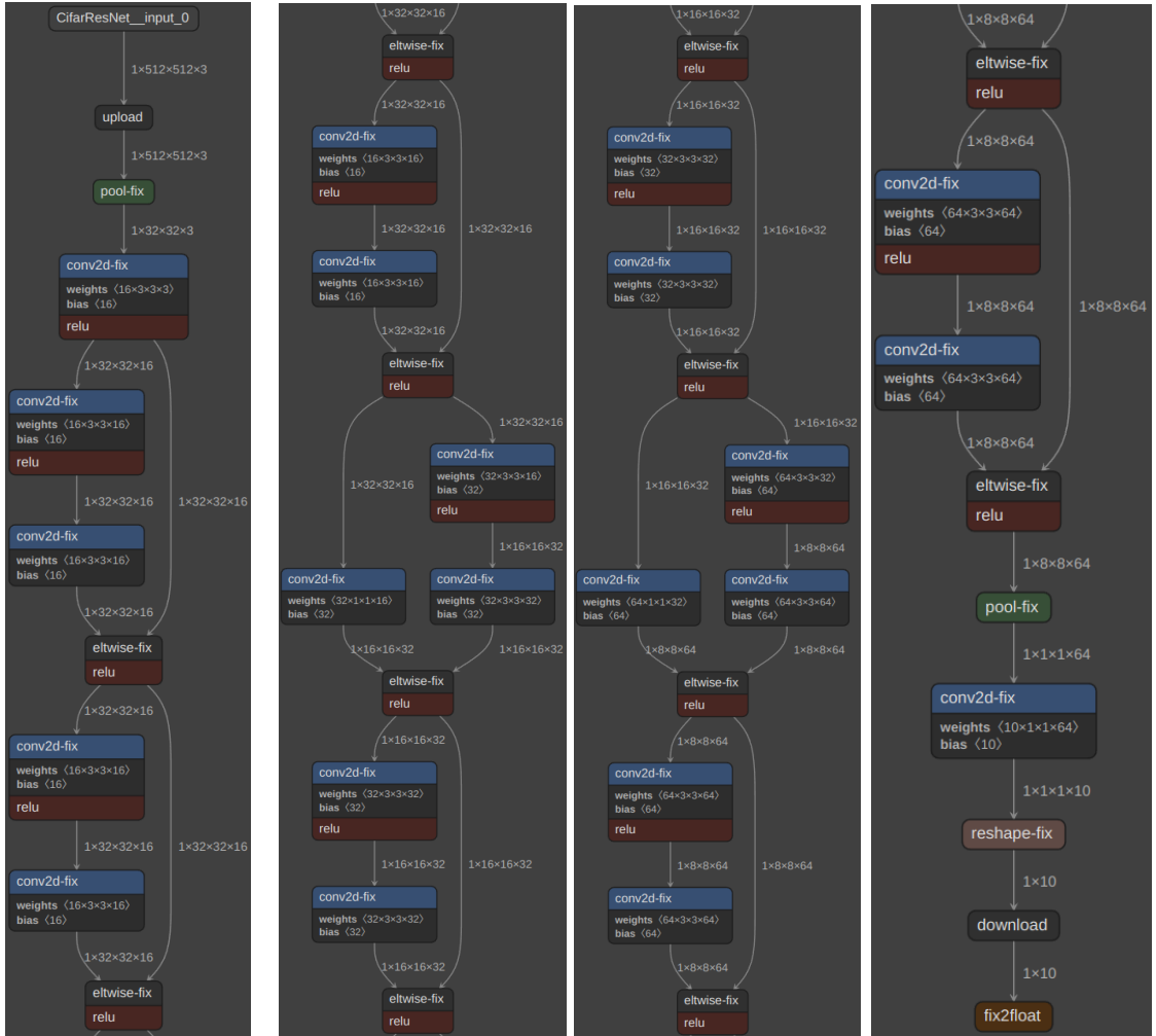
FIGURE 5.2: ResNet-20 Layer Structures Accepting a 512x512 Image after Modifications
