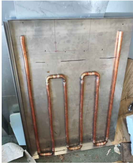
Figure 40: The container and the copper pipes of the PVT PCM system
