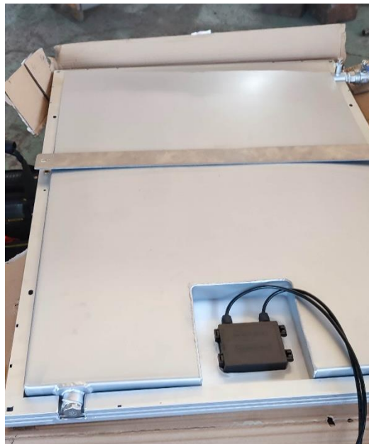
Figure 43: Container and piping system attached to the back of the PV (backside)
