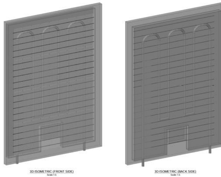
Figure 39: Front and backside of the Photovoltaic Thermal PCM system
